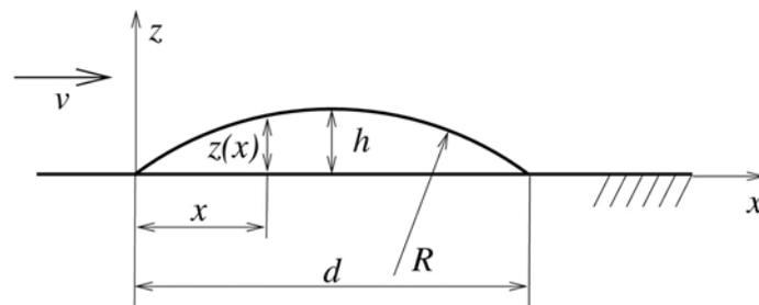
Fig. 5. The standardized artificial obstacle
