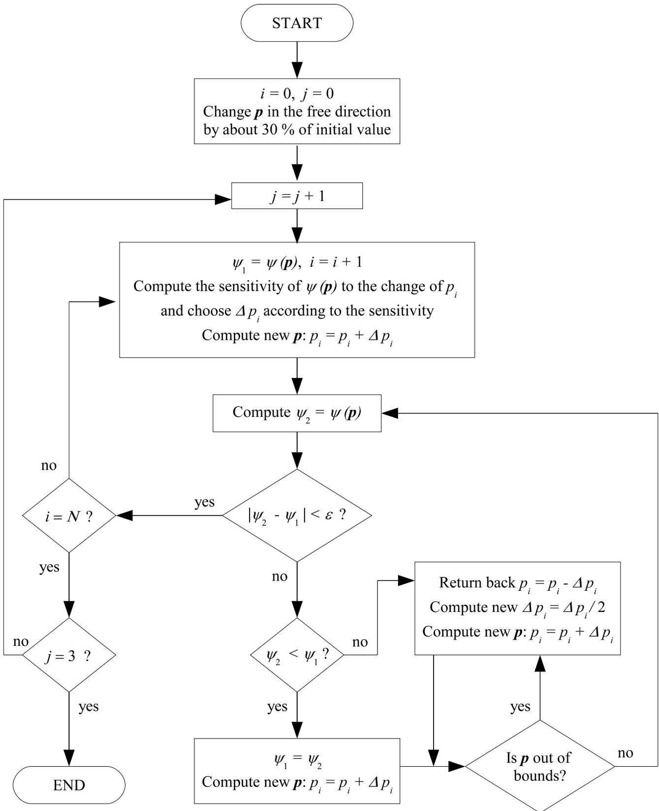
Fig. 7. The optimization methodology for the design of the APCS characteristics for the given bus weight
