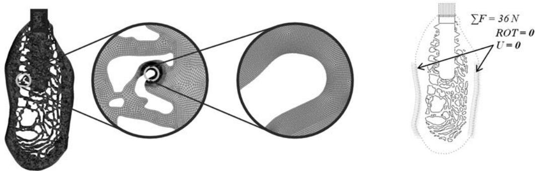
Fig. 7. FE mesh and the boundary conditions (model with the implant)
