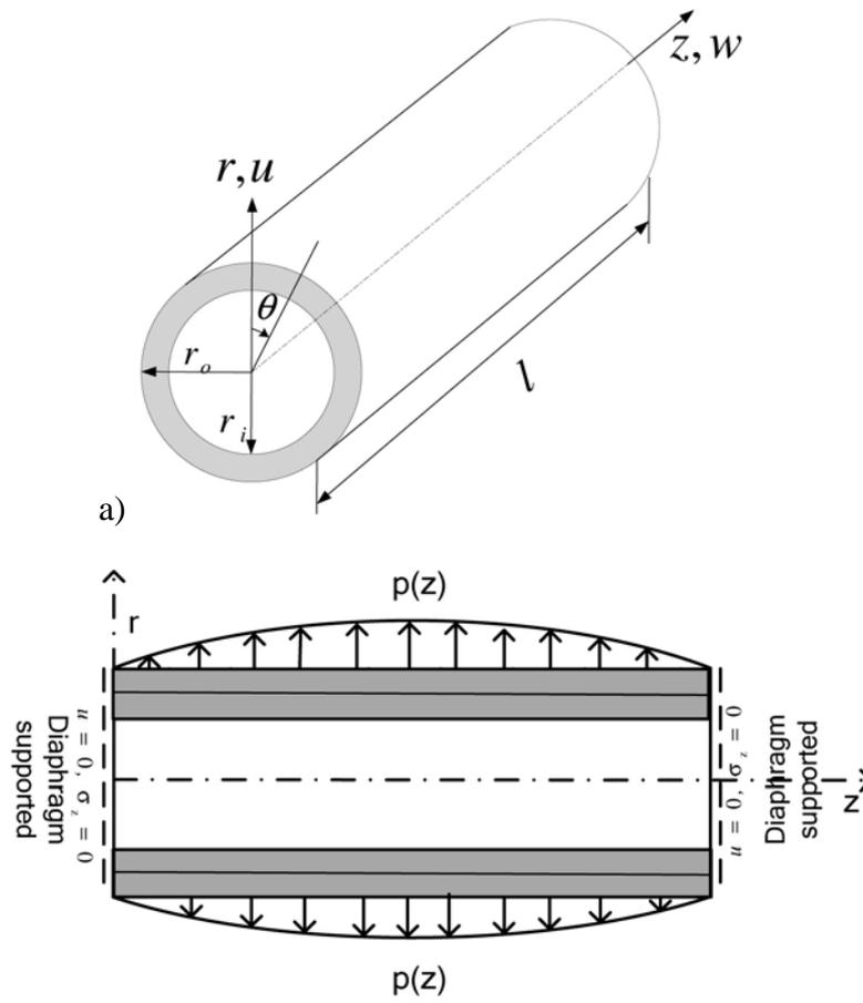
Fig. 1. a) Coordinate system and geometry of cylinder, b) finite cylinder under sinusoidal external pressure loading
