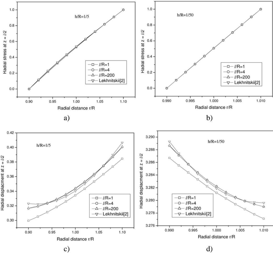
Fig. 2. Distribution of radial stress  $\bar{\sigma}_r$  and radial displacement  $\bar{u}$  through thickness subjected to sinusoidal loading for orthotropic cylinder
