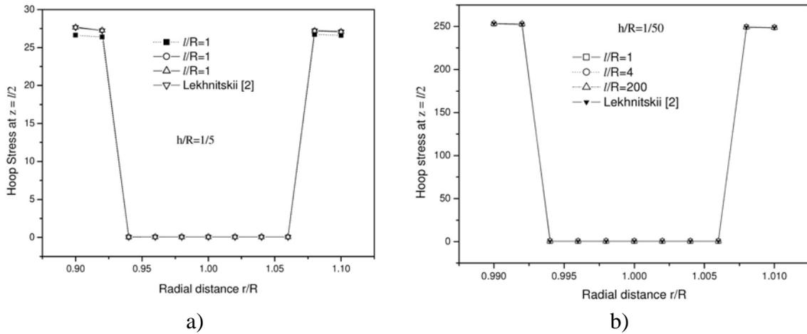
Fig. 9. Distribution of hoop stress  $\overline{\sigma_\theta}$  through thickness subjected to sinusoidal loading for sandwich cylinder
