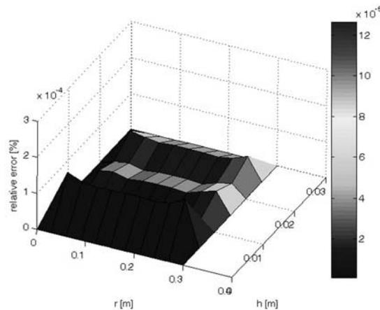
Fig. 4. Relative nodal error distribution over discretized plate
