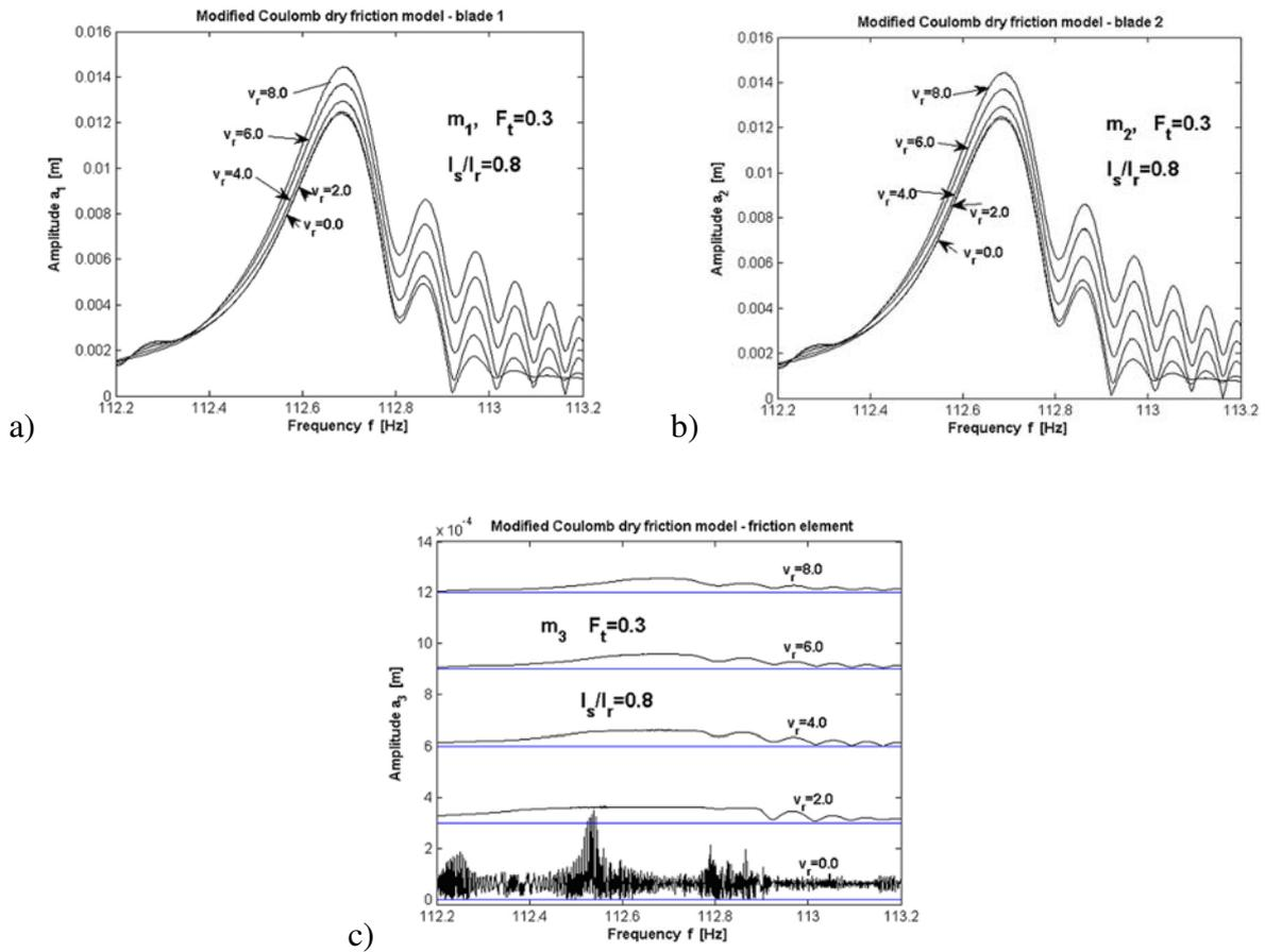
Fig. 14. Influence of different critical velocity  $v_r$  at  $F_T = 0.3$  and at ratio  $l_s/l_r = 0.8$
