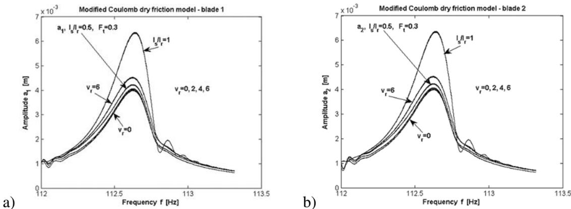
Fig. 10. Influence of critical velocity  $v_r$  at  $F_T = 0.3$  and at ratio  $l_s/l_r = 0.5$
