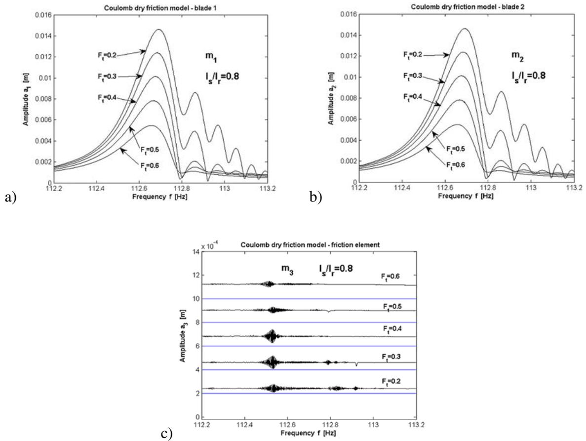
Fig. 13. Influence of different dry friction forces  $F_T = 0.2\text{--}0.6$  at  $l_s/l_r = 0.8$
