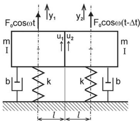
Fig. 3. Mathematical model of two blades system with direct friction contact
