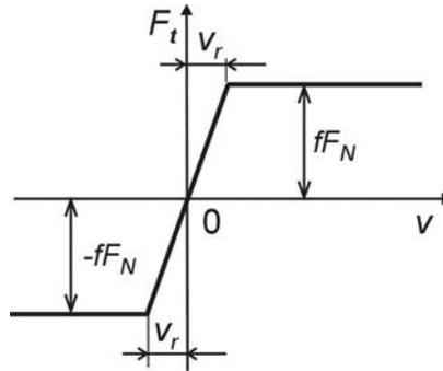
Fig. 4. Modified Coulomb friction characteristics
