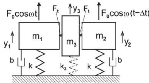
Fig. 11. Mathematical model of two blades system with friction element
