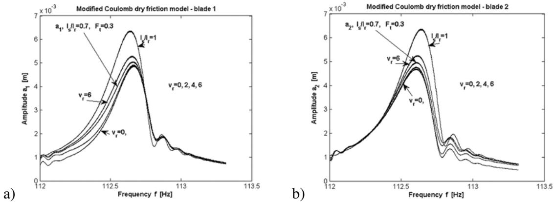
Fig. 9. Influence of critical velocity  $v_r$  at  $F_T = 0.3$  and at ratio  $l_s/l_r = 0.7$
