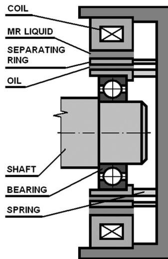
Fig. 4. Scheme of the damping device
