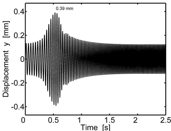
Fig. 18. Rotor displacement time history – variant 1
