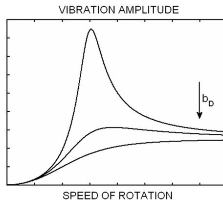
Fig. 3. Rotor frequency responses
