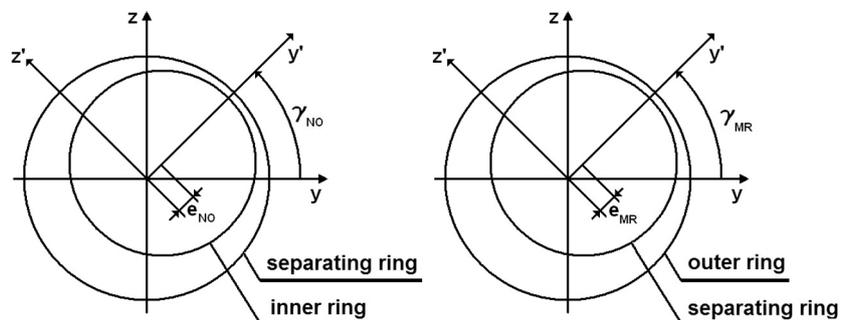
Fig. 5. The damper's coordinate systems
