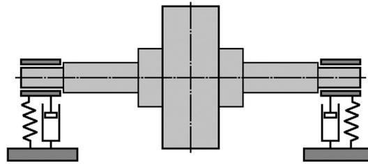
Fig. 1. Scheme of the simplified rotor system
