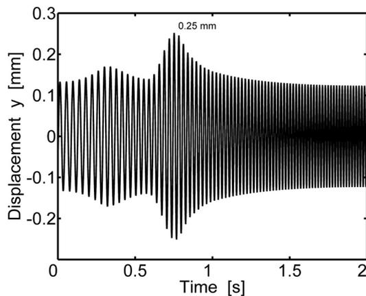
Fig. 26. Rotor displacement time history – variant 3
