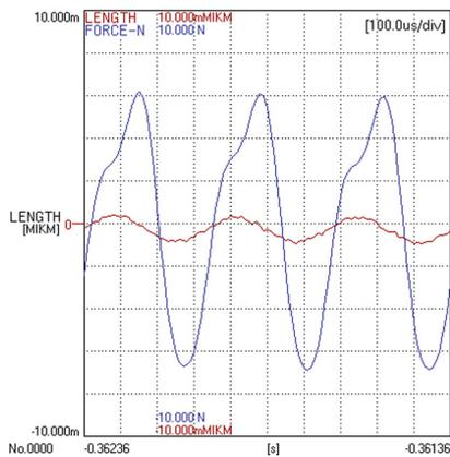
Fig. 18. Motion and friction force at 2 850 Hz
