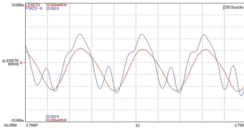
Fig. 14. Motion and friction force at 1 790 Hz
