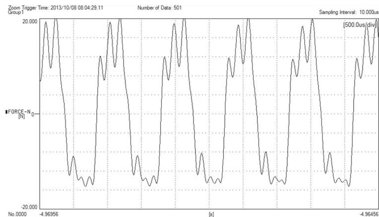
Fig. 2. Distortion of friction force record
