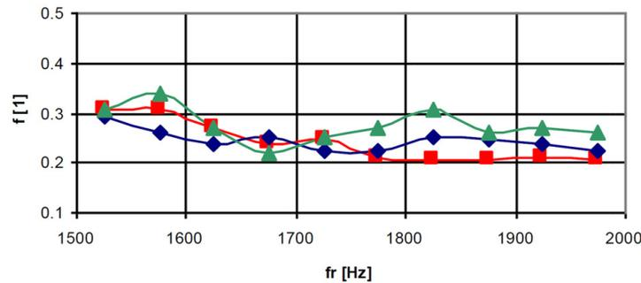
Fig. 12. Friction coefficient  $f$  in frequency range 1.5–2 kHz, contact pressure 462.48 N/m
