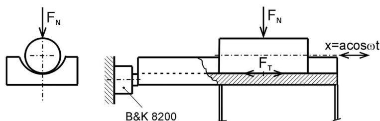
Fig. 5. Friction couple for high frequency measurements
