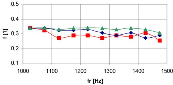
Fig. 6. Dry friction coefficient  $f$  in frequency range 1–1.5 kHz, contact pressure  $p = 231.24$  N/m
