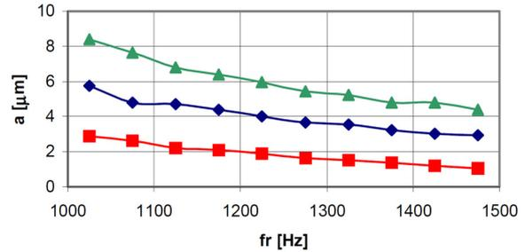
Fig. 7. Amplitudes of relative vibrations,  $I = 2, 4, 6$  A, ( $\square, \triangle, \diamond$ )
