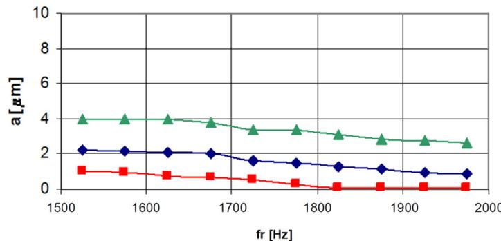
Fig. 13. Amplitudes of relative vibrations in frequency range 1.5–2 kHz
