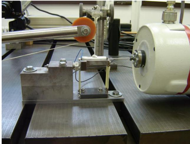
Fig. 1. Experimental set for dry friction measurements
