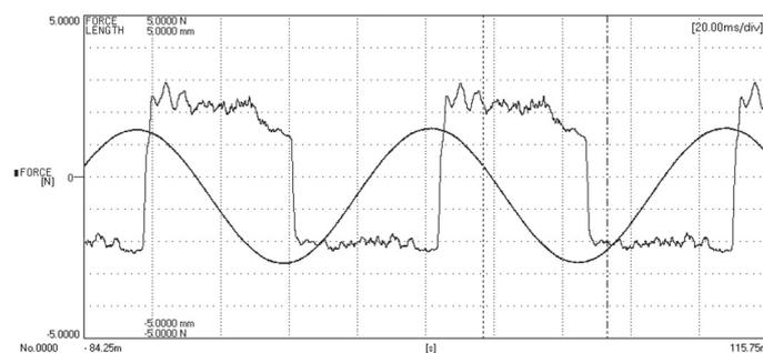
Fig. 3. Harmonic motion and friction force at 12 Hz
