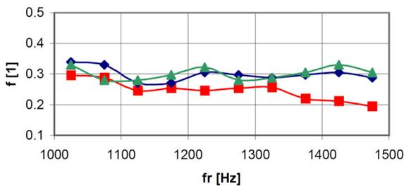
Fig. 8. Dry friction coefficient  $f$  in frequency range 1–1.5 kHz, contact pressure 462.48 N/m
