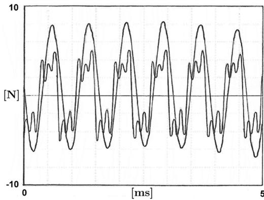
Fig. 10. Motion and friction force at 1249 Hz
