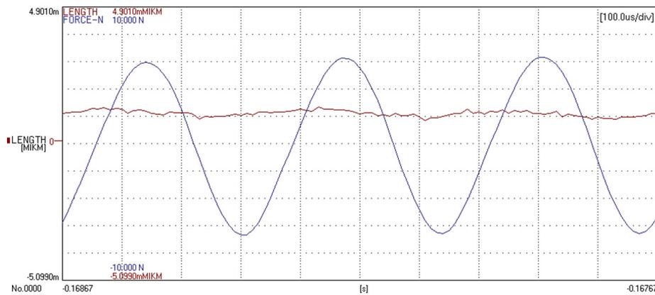
Fig. 20. Motion and friction force at 2950 Hz
