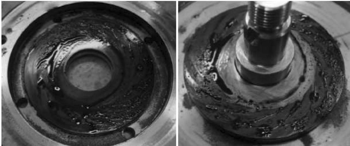
Fig. 26. Main thrust bearing and thrust disk polluted by the mixture of oil and graphite particles
