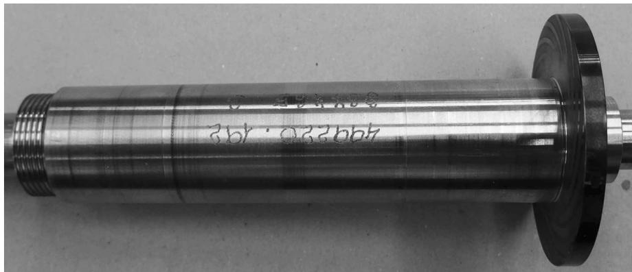
Fig. 29. Cleaned rotor
