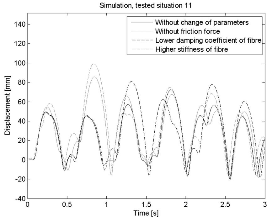
Fig. 15. Time histories of the weight displacement at “quicker” tested situation 11, influence of model parameters
