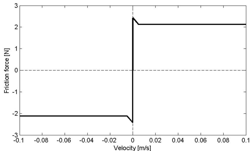
Fig. 4. Friction force acting between the weight and the prismatic linkage
