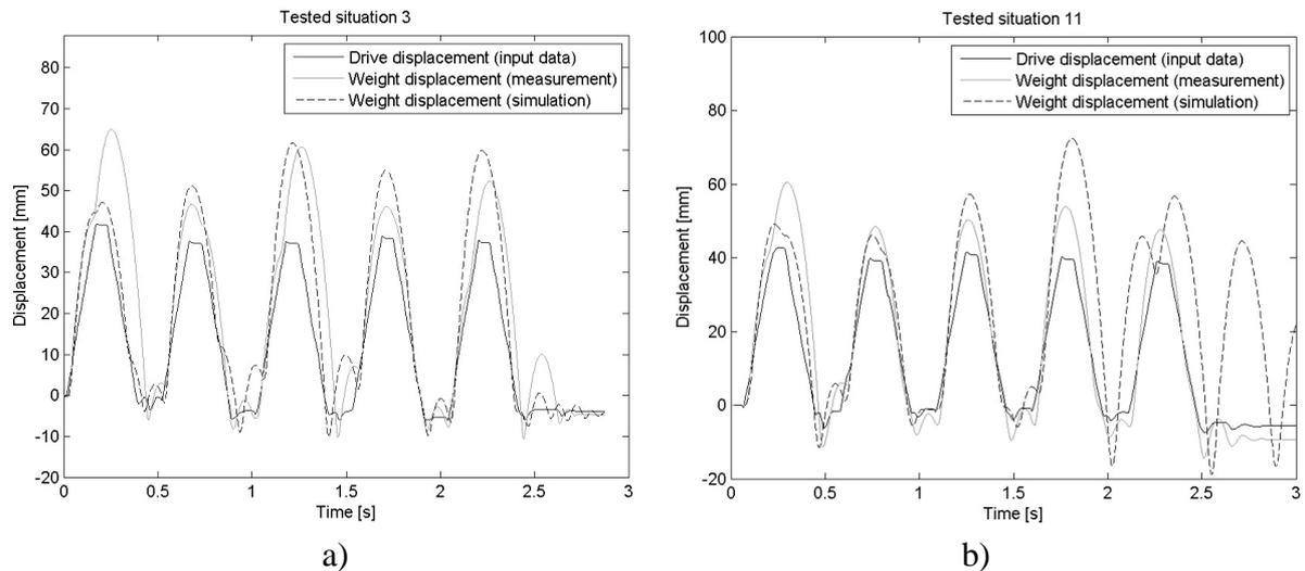
Fig. 8. Time histories of the weight displacement at “quicker” tested situations, influence of the mass of the weight, a) situation 3 (weight without added mass — taken from [21]), b) situation 11 (weight with added mass)
