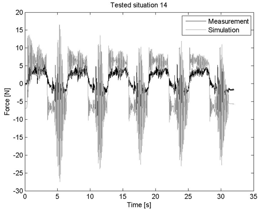
Fig. 7. Time histories of the dynamic force acting in a fibre at “slower” tested situation 14
