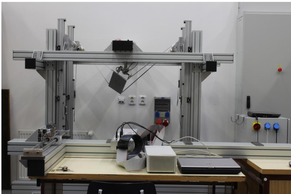
Fig. 2. The QuadroSphere spherical tilting mechanism
