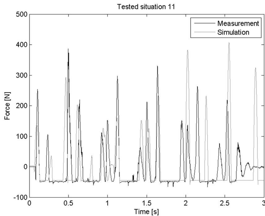
Fig. 10. Time histories of the dynamic force acting in a fibre at “quicker” tested situation 11, weight with added mass, influence of the mass of the weight
