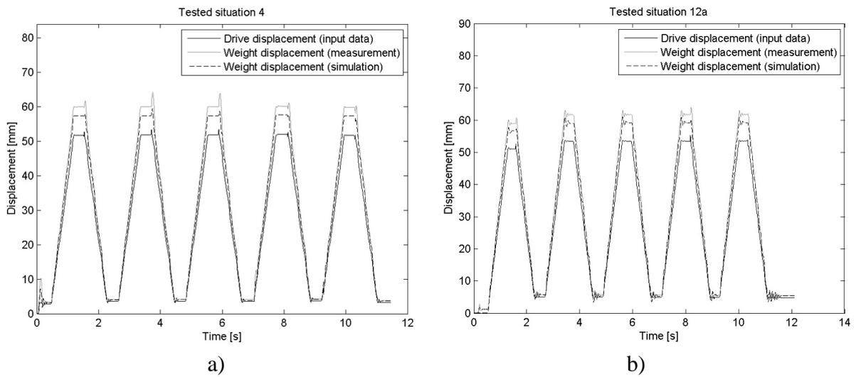
Fig. 11. Time histories of the weight displacement at “slower” tested situations, influence of the mass of the weight, a) situation 4 (weight without added mass — taken from [21]), b) situation 12a (weight with added mass)
