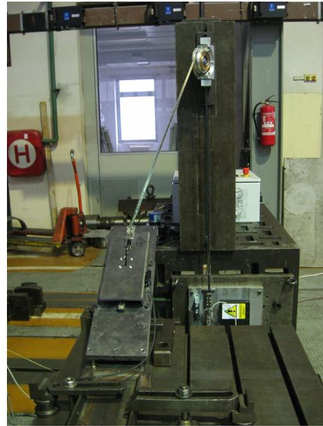
Fig. 1. Scheme and a real weight-fibre-pulley-drive mechanical system with asymmetric position of the weight
