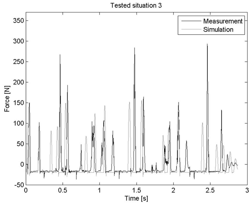
Fig. 9. Time histories of the dynamic force acting in a fibre at “quicker” tested situation 3, weight without added mass (taken from [21]), influence of the mass of the weight
