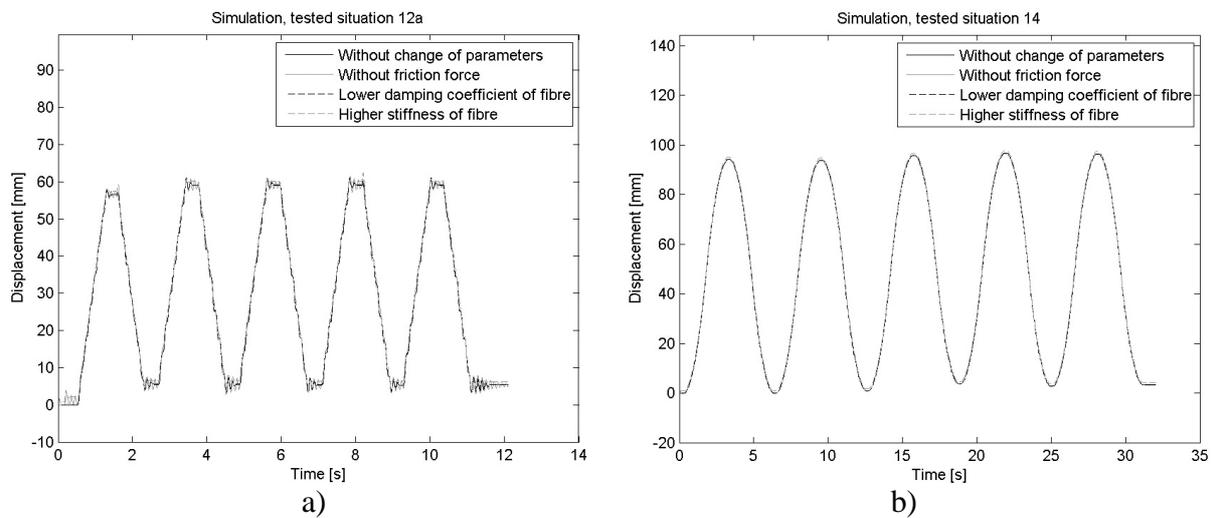
Fig. 16. Time histories of the weight displacement at “slower” tested situations, influence of model parameters, a) situation 12a, b) situation 14
