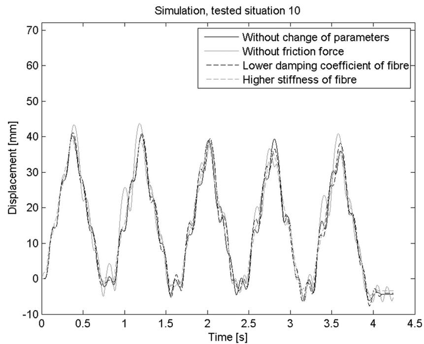
Fig. 14. Time histories of the weight displacement at “quicker” tested situation 10, influence of model parameters
