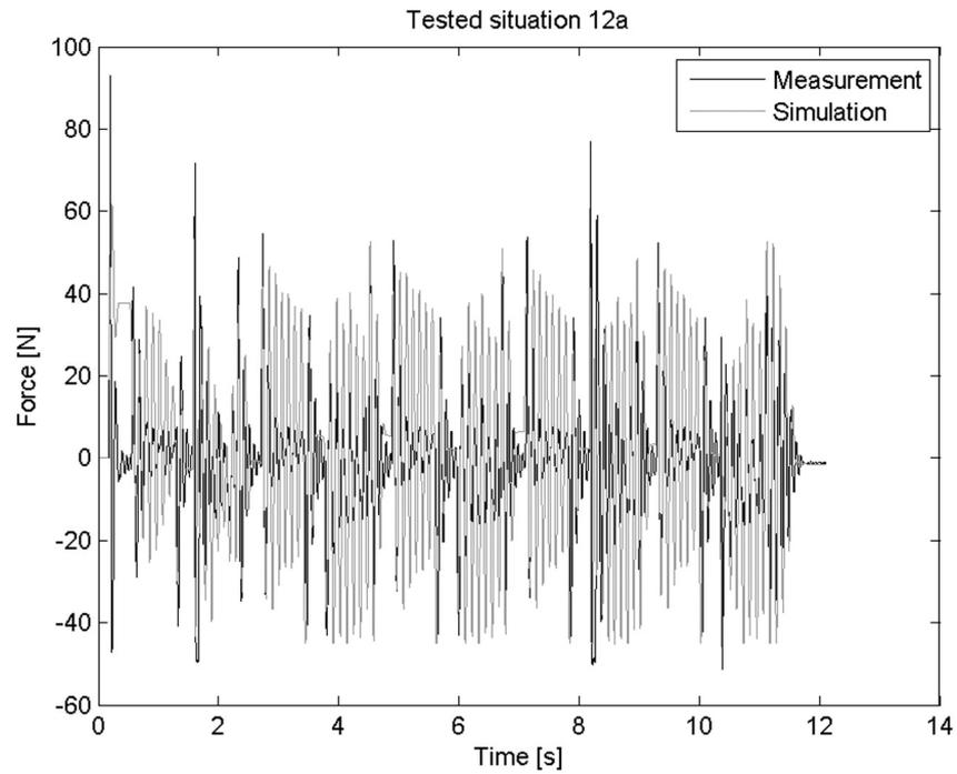
Fig. 13. Time histories of the dynamic force acting in a fibre at “slower” tested situation 12a, weight with added mass, influence of the mass of the weight
