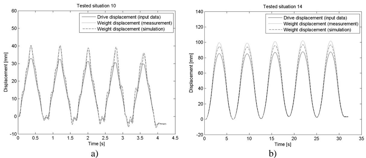
Fig. 5. Time histories of the weight displacement, a) at “quicker” tested situation 10, b) at “slower” tested situation 14
