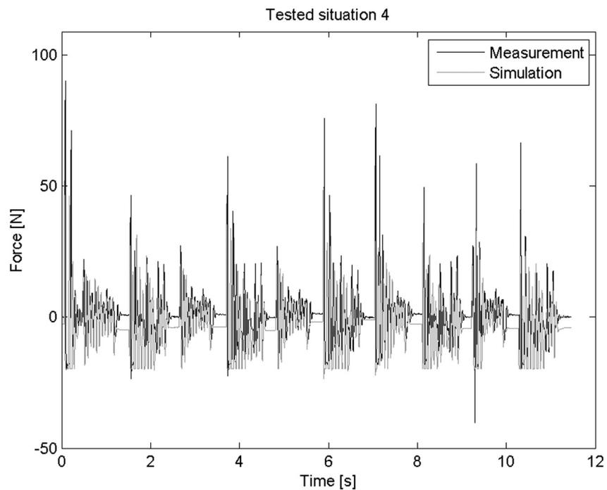
Fig. 12. Time histories of the dynamic force acting in a fibre at “slower” tested situation 4, weight without added mass (taken from [21]), influence of the mass of the weight
