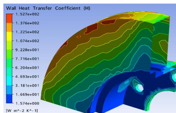
Fig. 9. Distribution of the heat transfer coefficient on a full disc in the steady-state case (FG 15)
