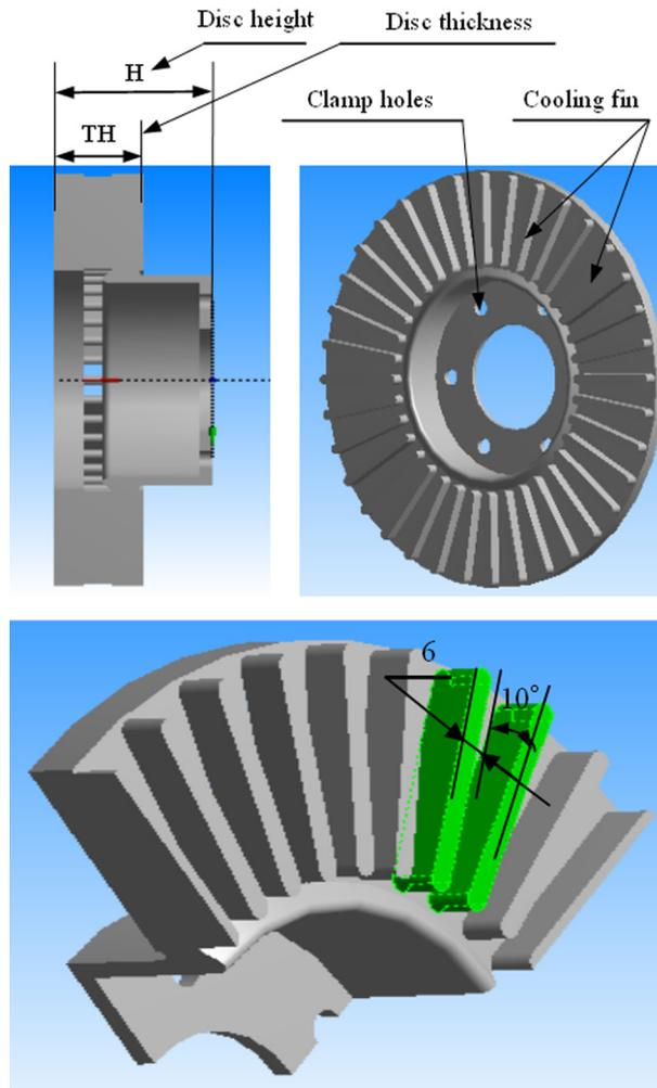
Fig. 1. Geometrical characteristics of the ventilated disc
