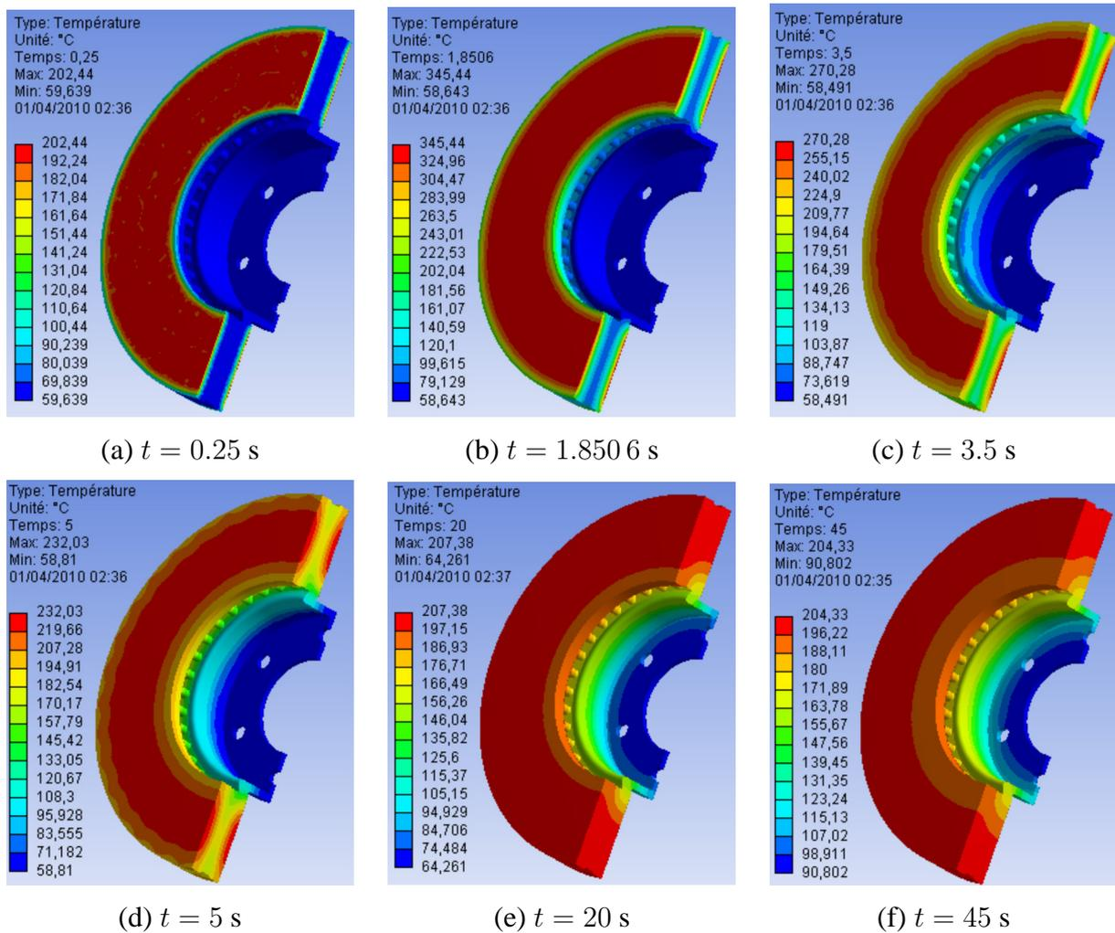
Fig. 22. Temperature distribution for the ventilated disc of material FG 15
