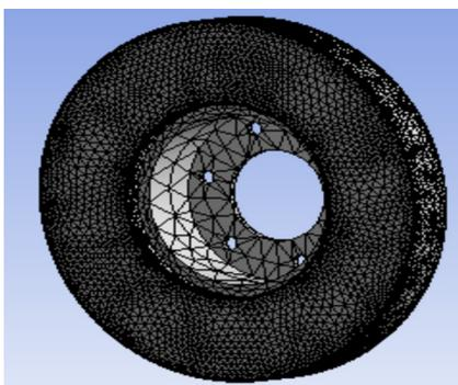
Fig. 14. Full type disc mesh model (total number of nodes 172 103 — total number of elements 114 421)
