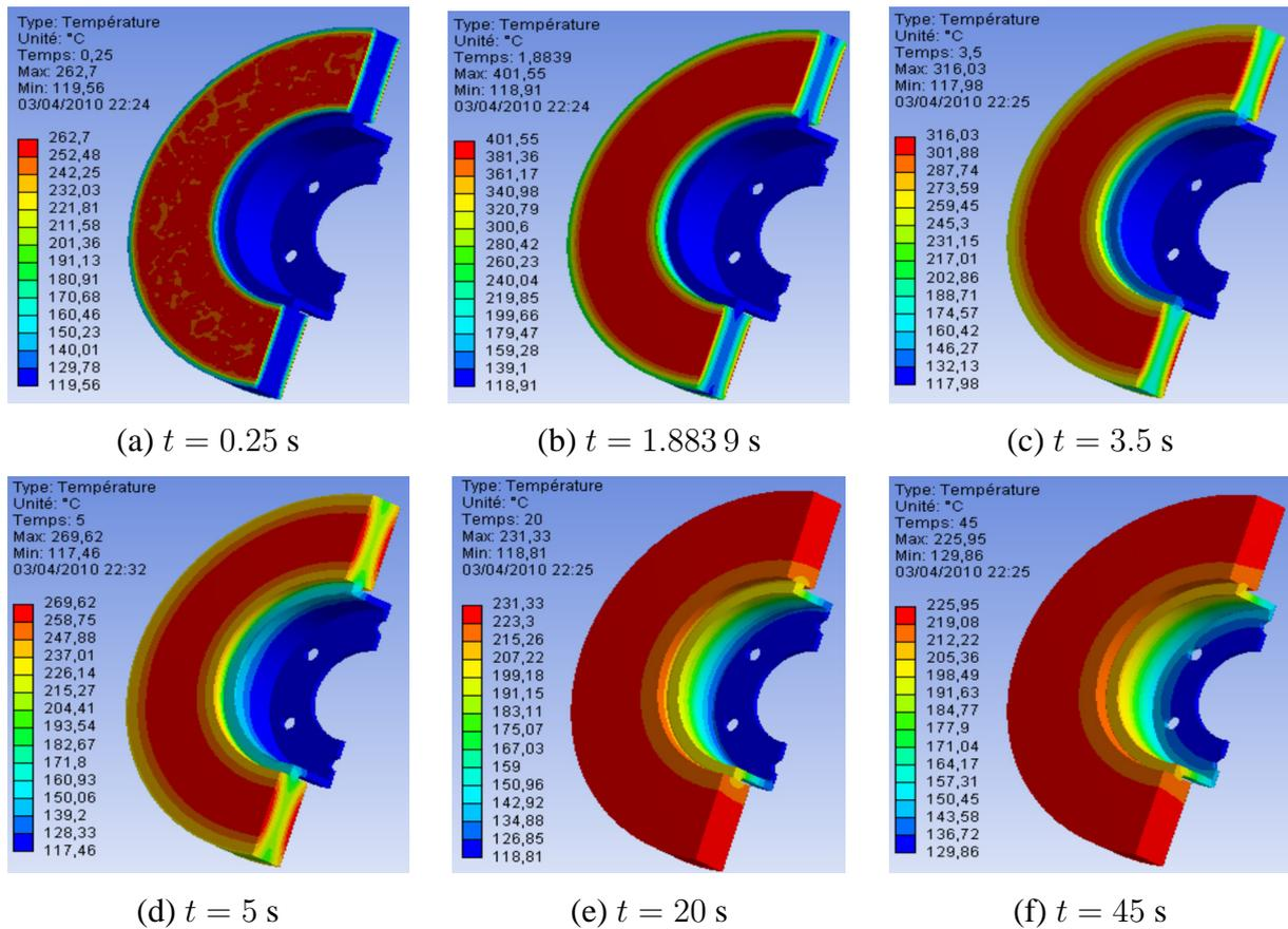
Fig. 19. Temperature distribution for the full disc of material FG 15
