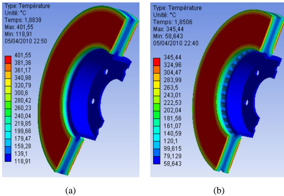
Fig. 16. Temperature distribution of a full (a) and ventilated disc (b) of cast iron (FG 15)
