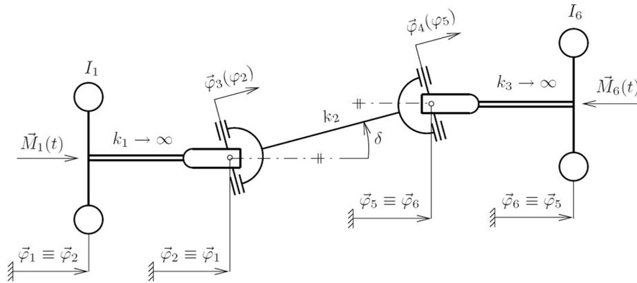
Fig. 1. Simplified scheme of Cardan shaft
