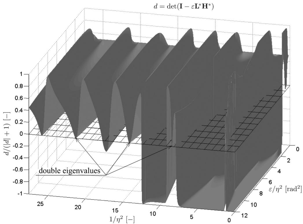
Fig. 3. Calculated values of determinant  $d$  in stable and unstable regions, problem without damping
