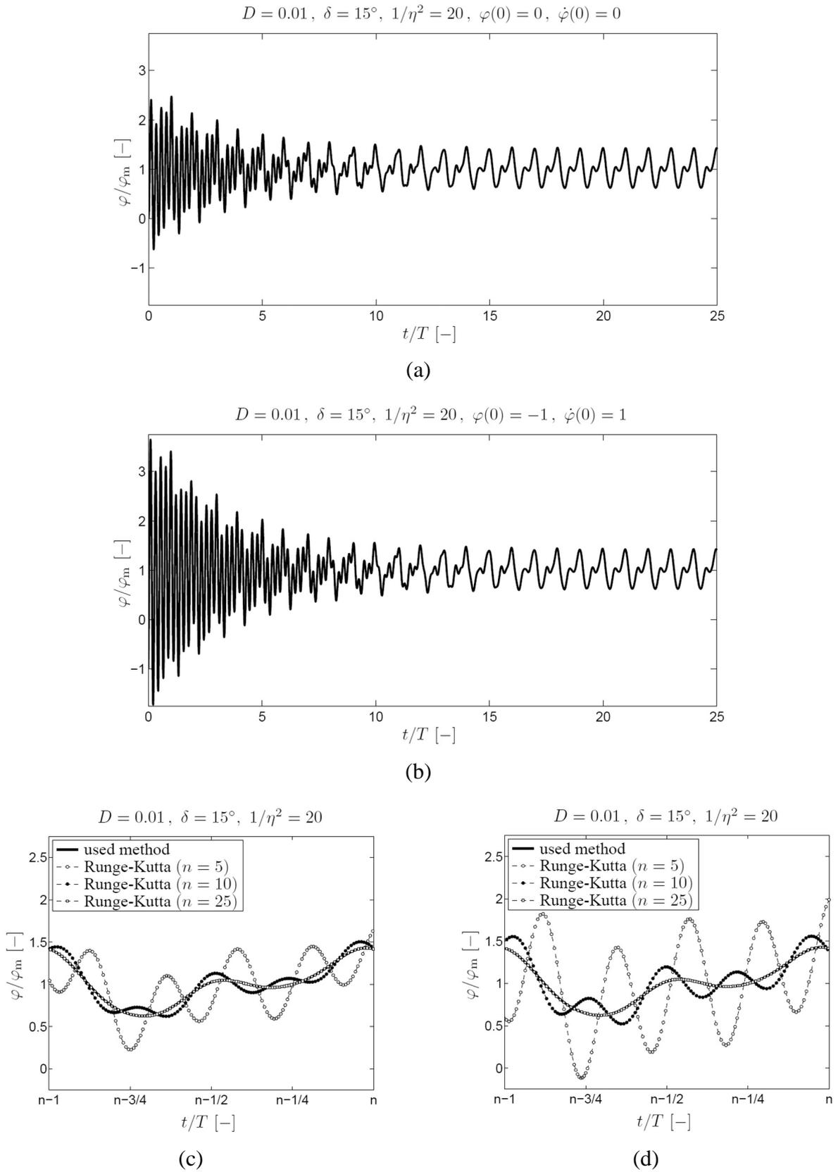
Fig. 8. Response calculated by the used method (c), (d), and the R-KI method (a)–(d) in a stable region: the R-KI method with homogeneous (a), (c), and inhomogeneous (b), (d) initial conditions; considered periodic term “ $-\varepsilon\varphi \cos 2\eta\tau$ ”
