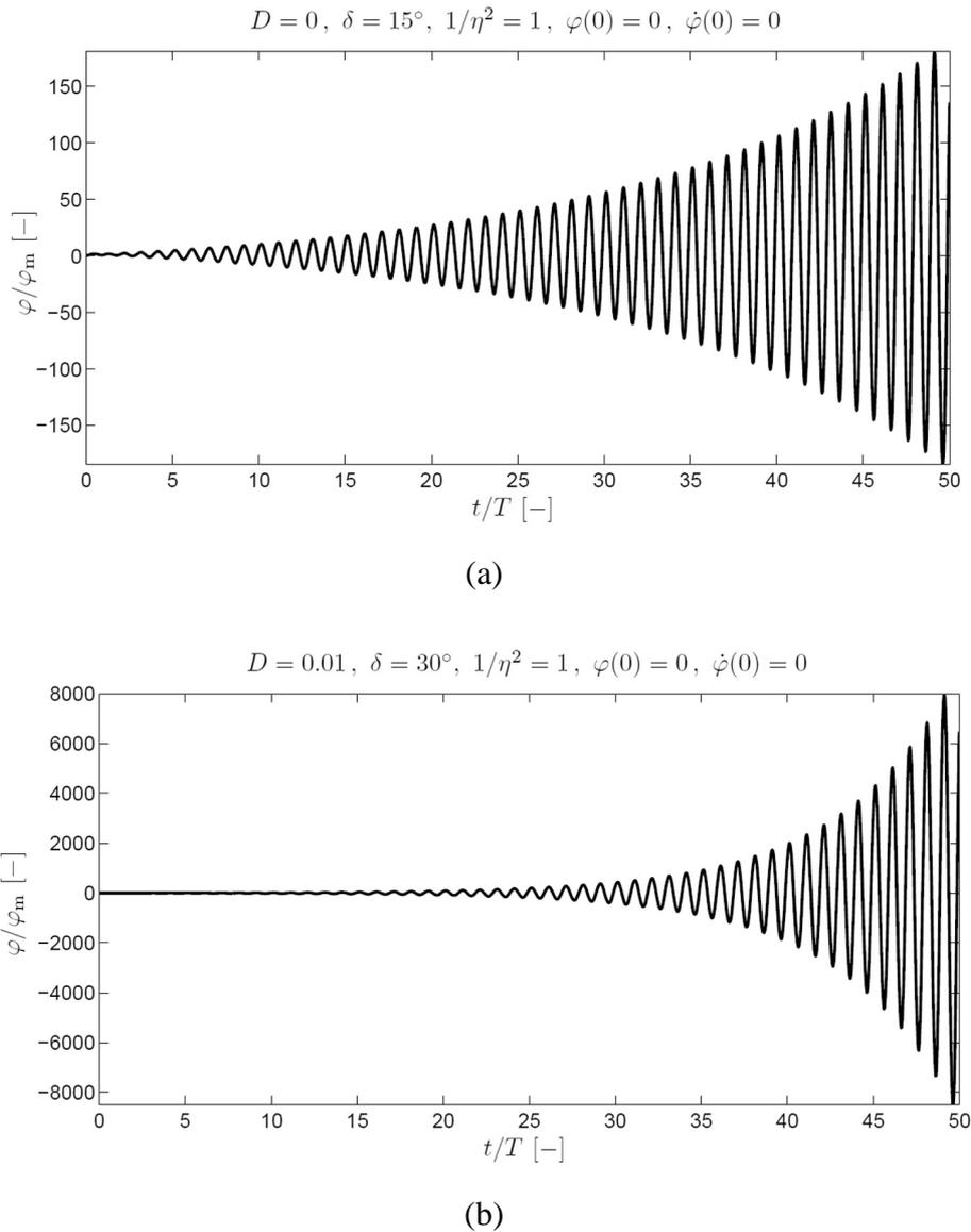
Fig. 5. Examples of calculation of response by the R-KI method in an unstable region
