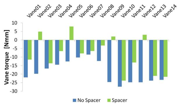
Fig. 22. Vane torque comparison: mid open (PR 4)
