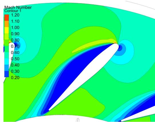
Fig. 31. Mach number contours: max open (PR 4)
