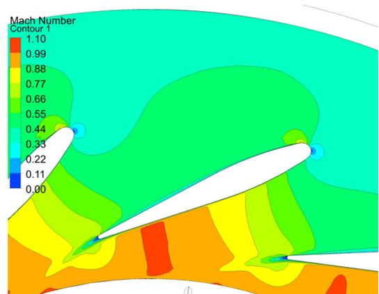
Fig. 20. Mach number contours: min open (PR 4)
