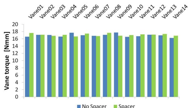
Fig. 13. Vane torque comparison: min open (PR 4)
