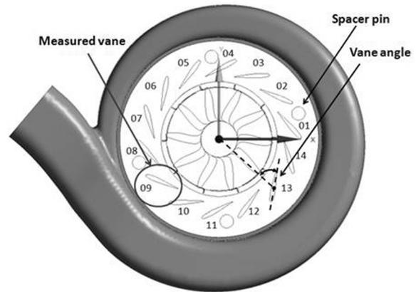
Fig. 4. Vane numbering & spacer pin positions
