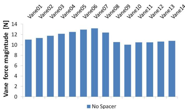
Fig. 15. Vane force distribution: mid open (PR 4)
