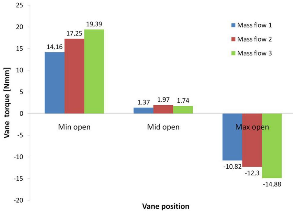
Fig. 43. Vane aero torque experimental results
