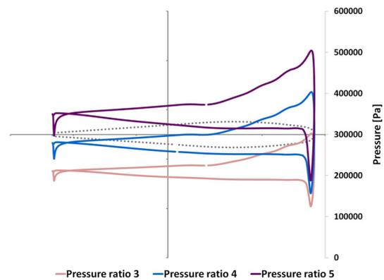
Fig. 29. Vane pressure distribution comparison
