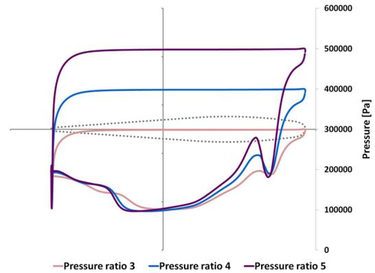
Fig. 9. Vane pressure distribution comparison
