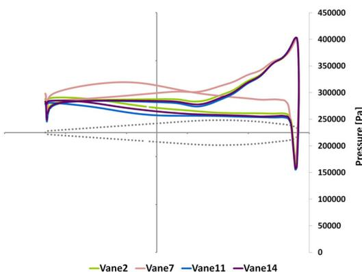
Fig. 28. Vane pressure distribution: max open (PR 4)
