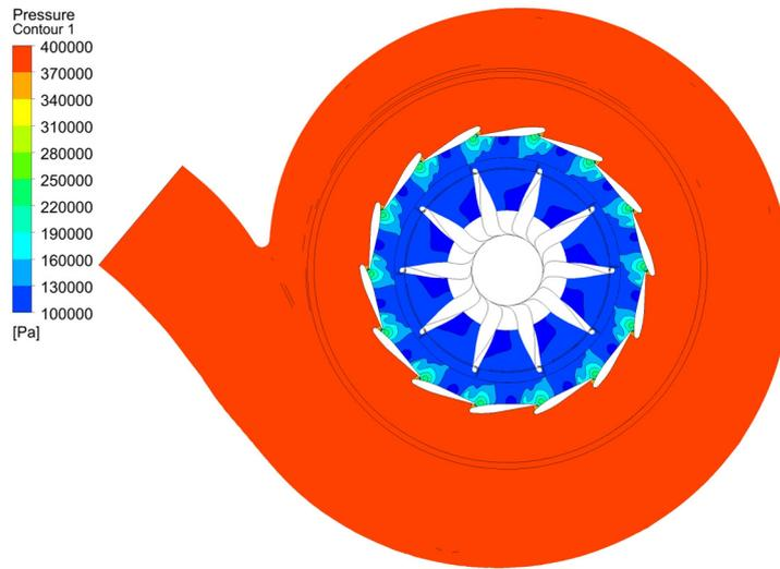
Fig. 5. Pressure contours: min open (PR 4)
