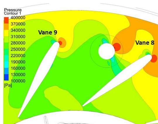
Fig. 35. Spacer pin pressure contours: max open (PR 4)
