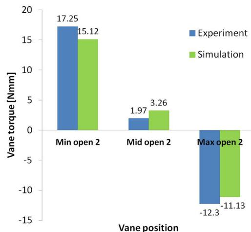
Fig. 45. Vane aero torque comparison (mass flow 2)
