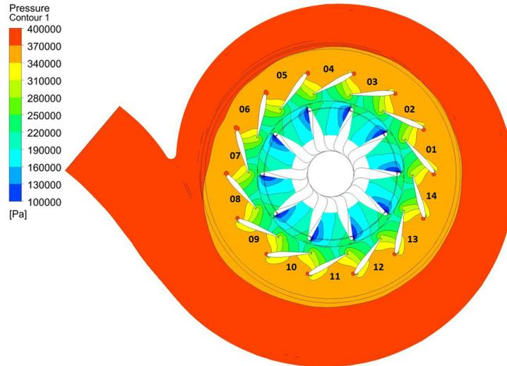
Fig. 14. Pressure contours: mid open (PR 4)
