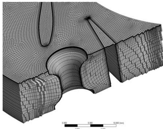
Fig. 2. Vane passage hexagonal grid with side clearance
