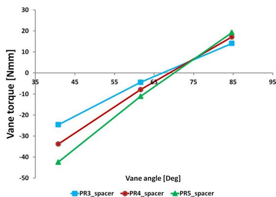
Fig. 39. Averaged vane torque vs. vane angle
