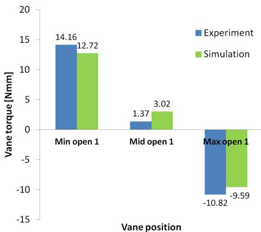
Fig. 44. Vane aero torque comparison (mass flow 1)
