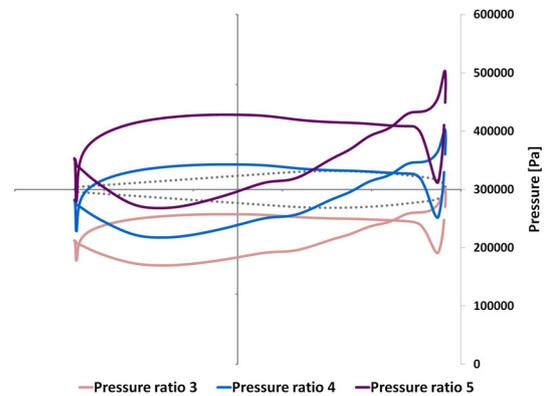
Fig. 18. Vane pressure distribution comparison
