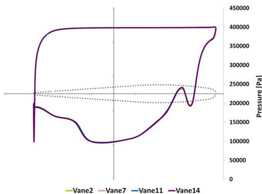
Fig. 8. Vane pressure distribution: min open (PR 4)
