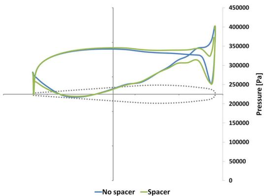
Fig. 23. Spacer pin influence: mid open (PR 4)
