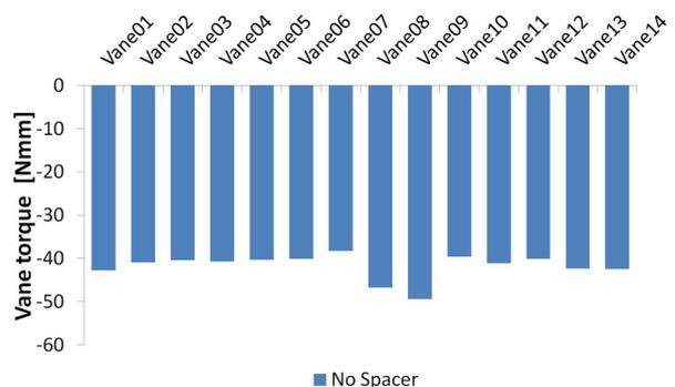
Fig. 27. Vane torque distribution: max open (PR 4)
