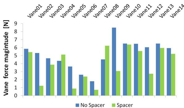
Fig. 32. Vane force comparison: max open (PR 4)
