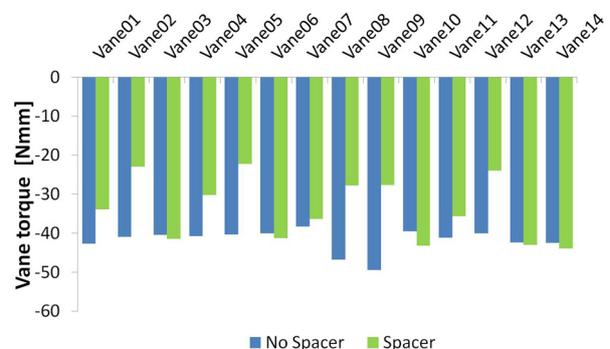
Fig. 33. Vane torque comparison: max open (PR 4)
