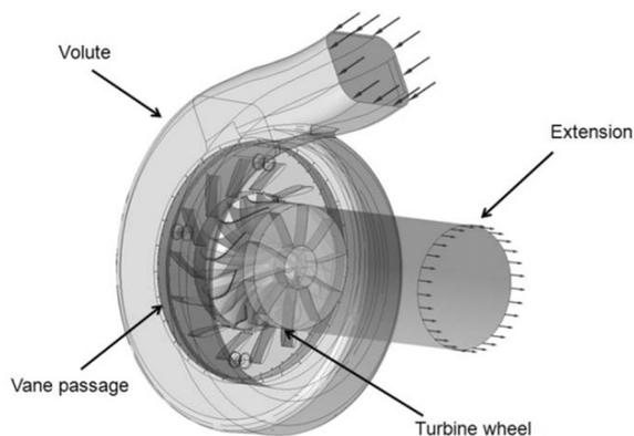
Fig. 1. Turbine stage geometry model
