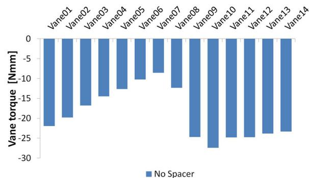
Fig. 16. Vane torque distribution: mid open (PR 4)
