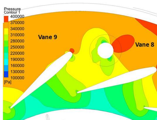
Fig. 24. Spacer pin pressure contours: mid open (PR 4)
