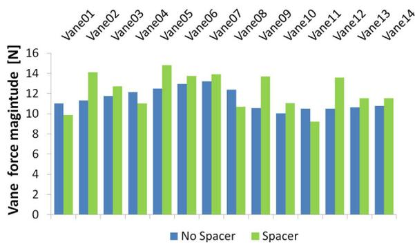
Fig. 21. Vane force comparison: mid open (PR 4)
