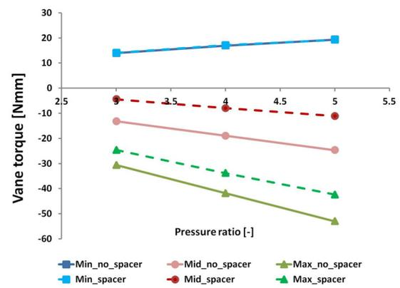
Fig. 37. Averaged vane torque vs. pressure ratio
