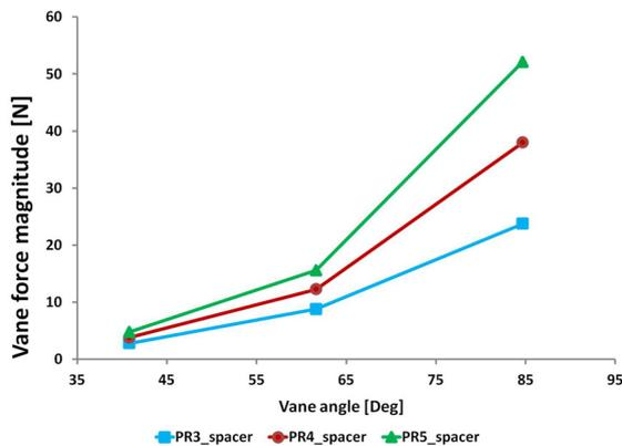
Fig. 38. Averaged vane force vs. vane angle
