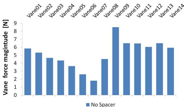
Fig. 26. Vane force distribution: max open (PR 4)
