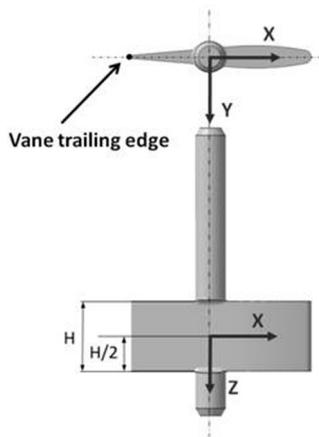
Fig. 3. Vane local coordinate system
