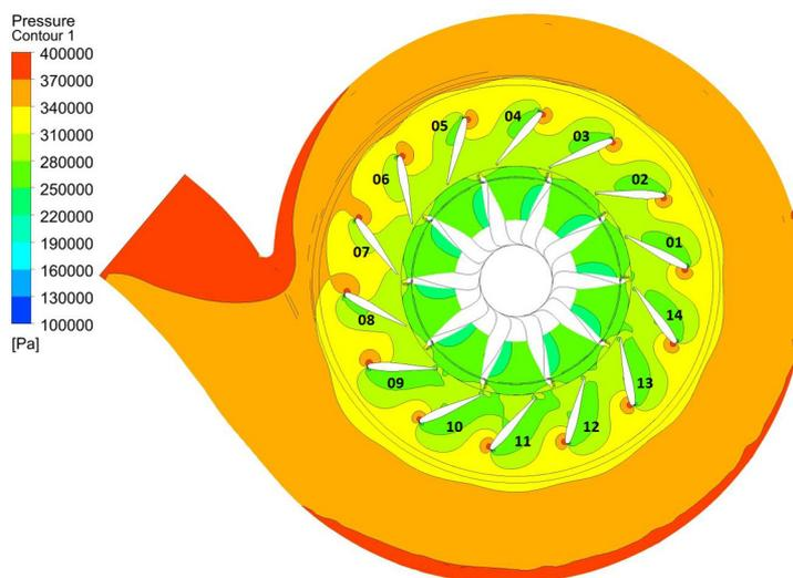
Fig. 25. Pressure contours: max open (PR 4)
