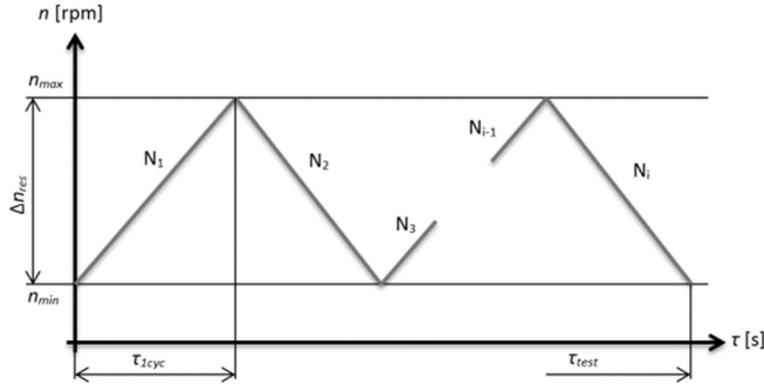
Fig. 8. Scheme of the vibration test program
