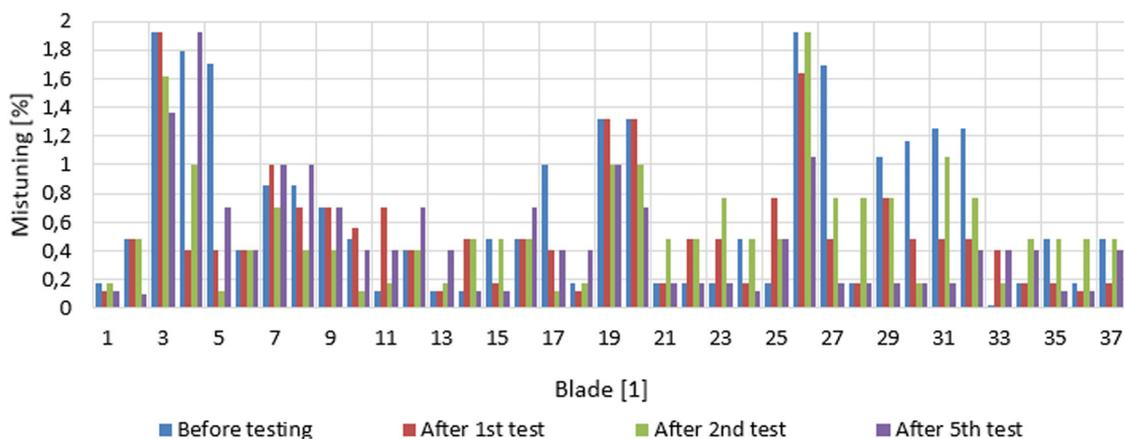
Fig. 12. Natural frequencies during testing
