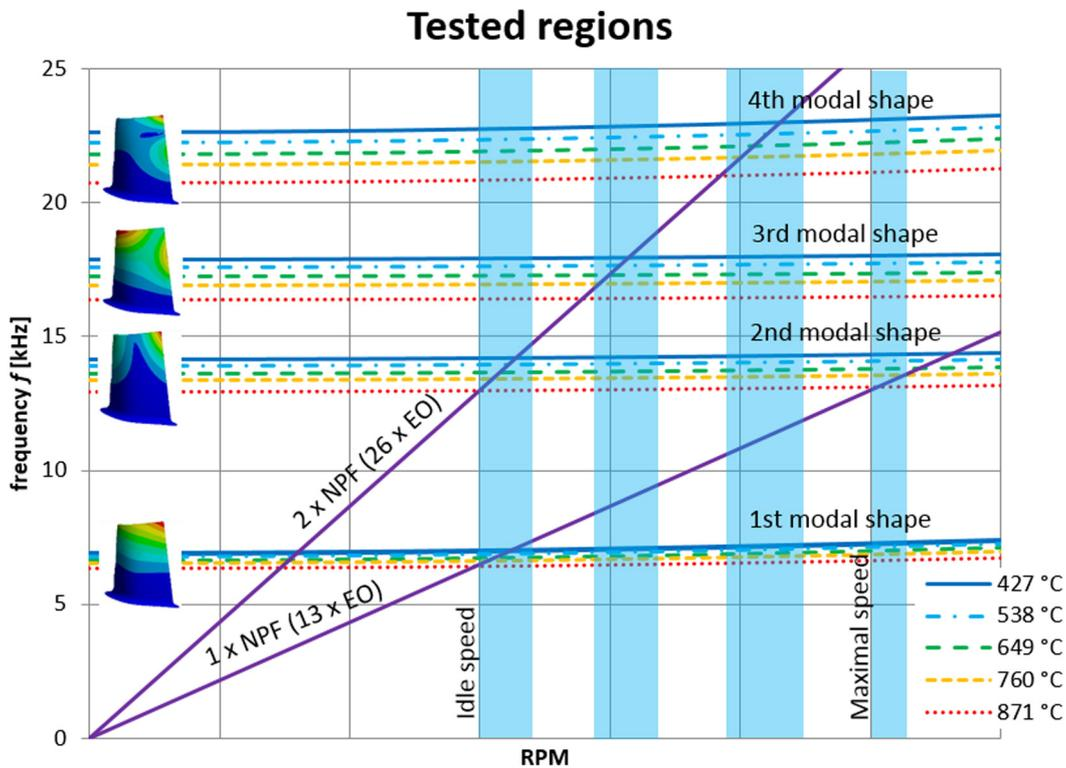
Fig. 9. Experimental regions for the verification of rotational speeds
