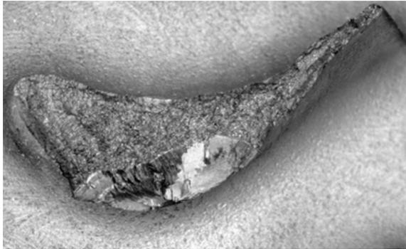
Fig. 10. Crack surface on the blade root
