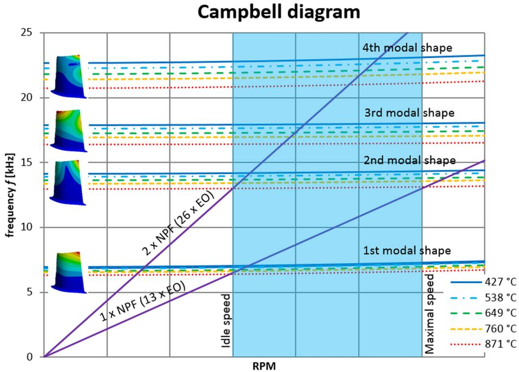
Fig. 3. Campbell diagram with the effect of temperature and centrifugal force
