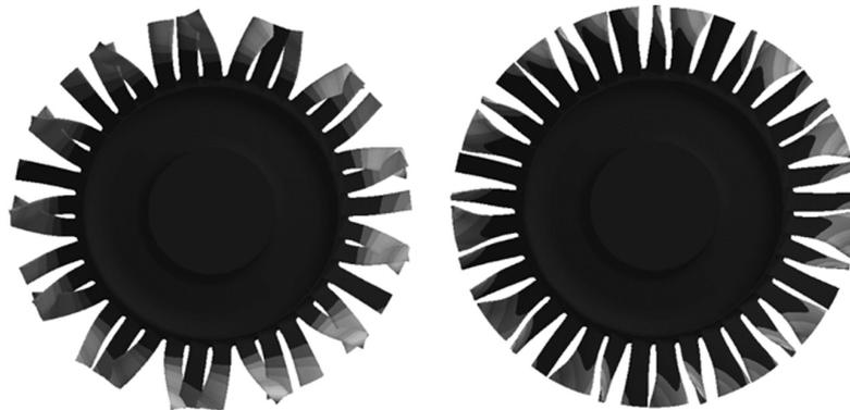
Fig. 4. Coupled vibration of the blisk (total displacement): (left) 1<sup>st</sup> modal shape with 13 nodal diameters, (right) 2<sup>nd</sup> modal shape with 13 nodal diameters
