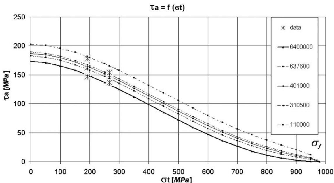
Fig. 3. Fuxa’s approximation for combined torsion – tension loading
