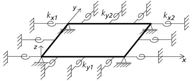
Fig. 1. Thin plate supported with torsional springs
