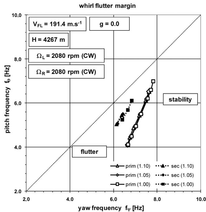
Fig. 7. Whirl flutter stability margins – symmetrical revolutions, identical directions of revolution (CW-CW), legend: prim = primary flutter ( $S\Theta/A\Psi$ ), sec = secondary flutter ( $A\Theta/S\Psi$ ), (1.xx) = VFR, HFR
