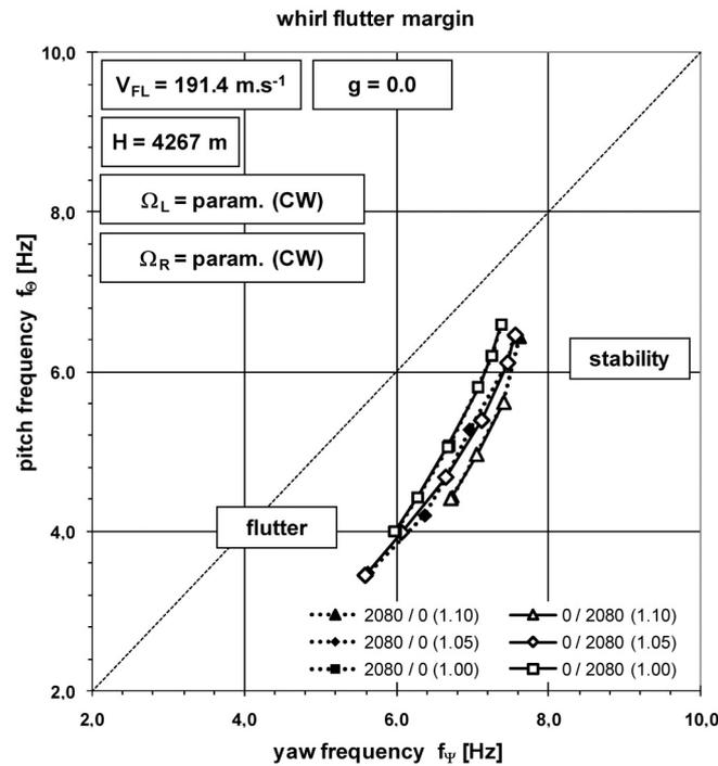
Fig. 11. Whirl flutter stability margins – a single rotor omission, legend:  $\Omega_L/\Omega_R$ , (1.xx) =  $VFR$ ,  $HFR$
