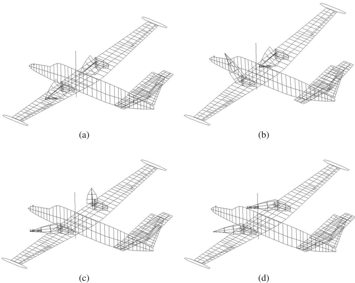
Fig. 6. Engine vibration modes: (a) symmetric pitch, (b) antisymmetric pitch, (c) symmetric yaw and (d) antisymmetric yaw
