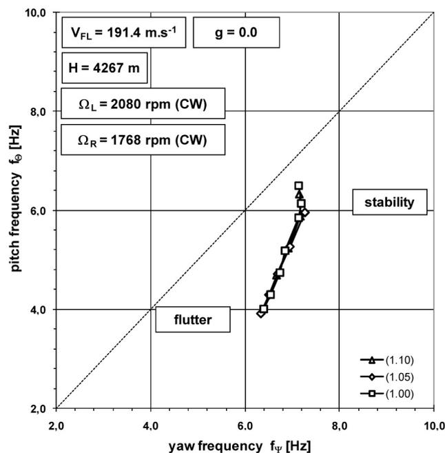
Fig. 12. Whirl flutter stability margins – unsymmetrical revolutions, reduced revolutions of a single rotor, identical directions of revolution (CW-CW), primary flutter only, legend: (1.xx) =  $VFR$ ,  $HFR$
