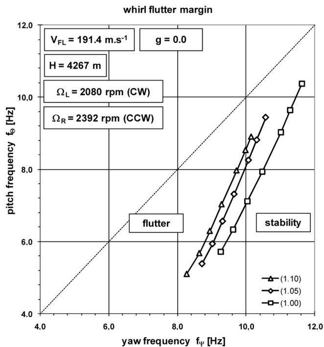
Fig. 15. Whirl flutter stability margins – unsymmetrical revolutions, increased revolutions of a single rotor, inverse directions of revolutions (CW-CCW), legend: (1.xx) = VFR, HFR
