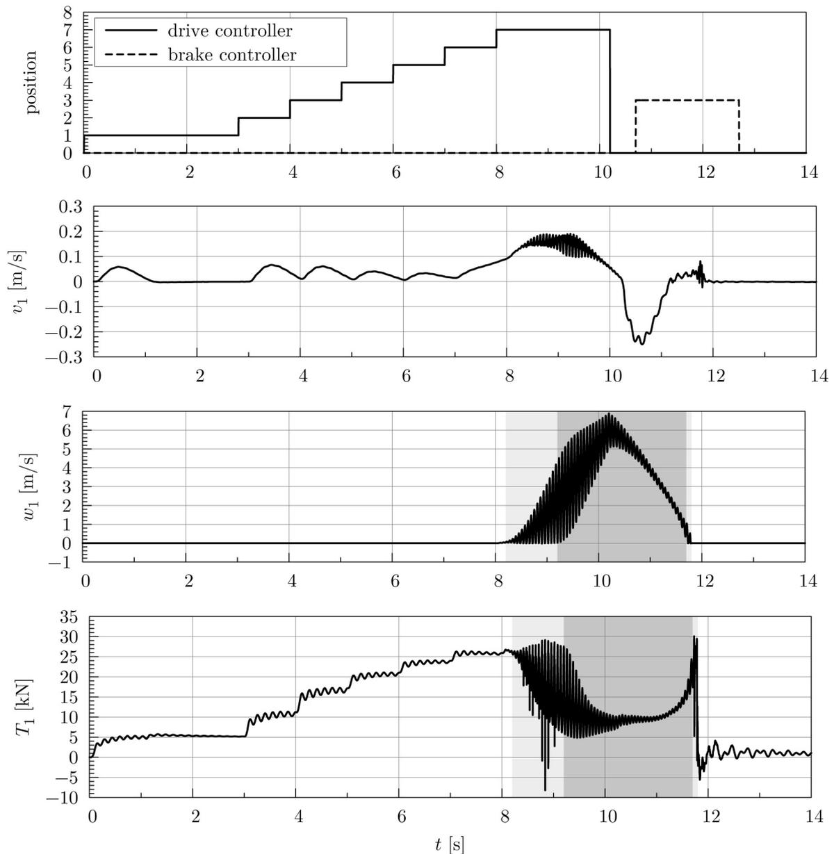
Fig. 8. Simulation results with the CFFM:  $v_1$  speed of forward motion,  $w_1$  creep velocity and  $T_1$  tangential force for the first wheelset. Lighter shaded areas indicate sliding with stick-slip effect, the area with darker shading means uninterrupted sliding
