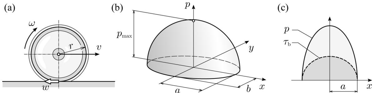
Fig. 1. Illustration to the wheel-rail contact problem: (a) movement of a wheel in a planar model, (b) distribution of pressure in Hertzian contact with  $a, b$  semiaxes of the contact ellipse, (c) longitudinal section of this distribution together with traction bound  $\tau_b$
