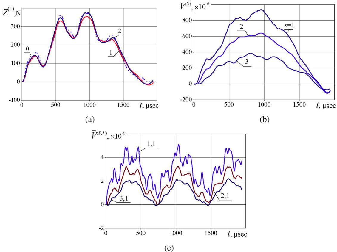
Fig. 9. Contact force identification based on experimental data: (a) configurations of true and identified loads; (b) strain vs. time; (c) “influence”/“transfer” functions (see Fig. 7c)
