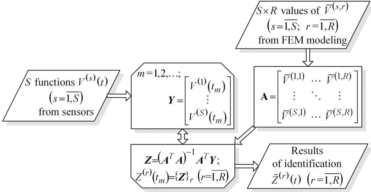
Fig. 2. Algorithm for loads identification for problem in the quasi-static statement
