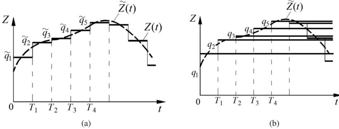
Fig. 3. Approximation of unknown dependencies by step functions: (a) representation as a piecewise constant function; (b) representation as a combination of step functions
