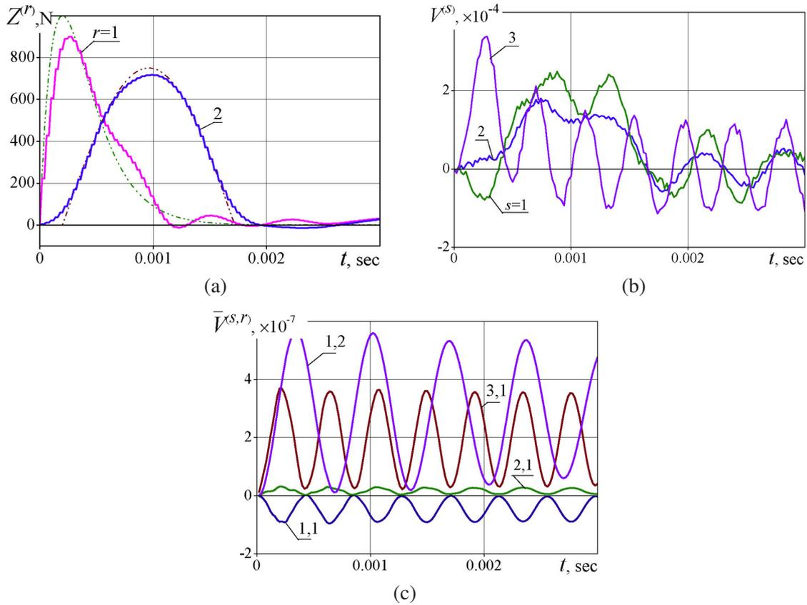
Fig. 7. Result of identification of non-stationary loads: (a) configurations of true and identified loads; (b) strain vs. time; (c) “influence”/“transfer” functions
