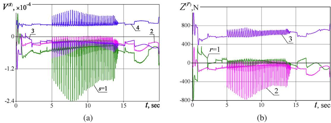
Fig. 6. Result of identification of quasi-static forces: (a) values of strain as input data; (b) values of identified loads
