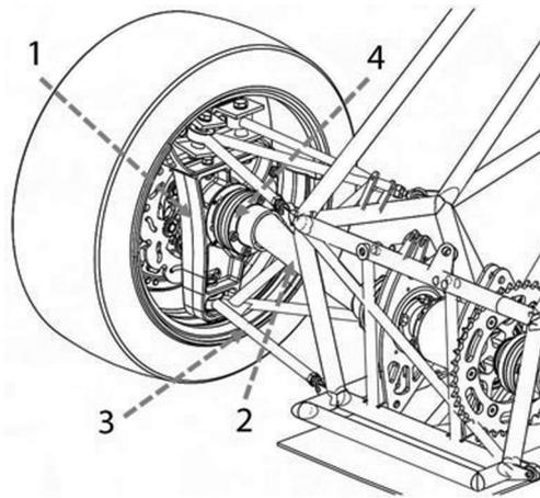
Fig. 1. Wheel suspension with gentelligent technology for measuring loads during the life cycle: 1 – wheel carrier; 2 – driving shaft; 3 – wishbone; 4 – bearing
