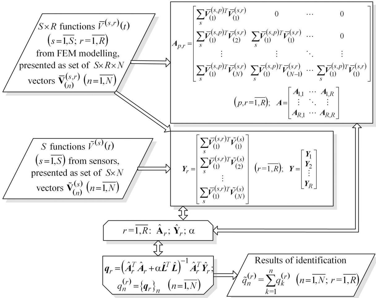
Fig. 4. Algorithm for non-stationary loads identification
