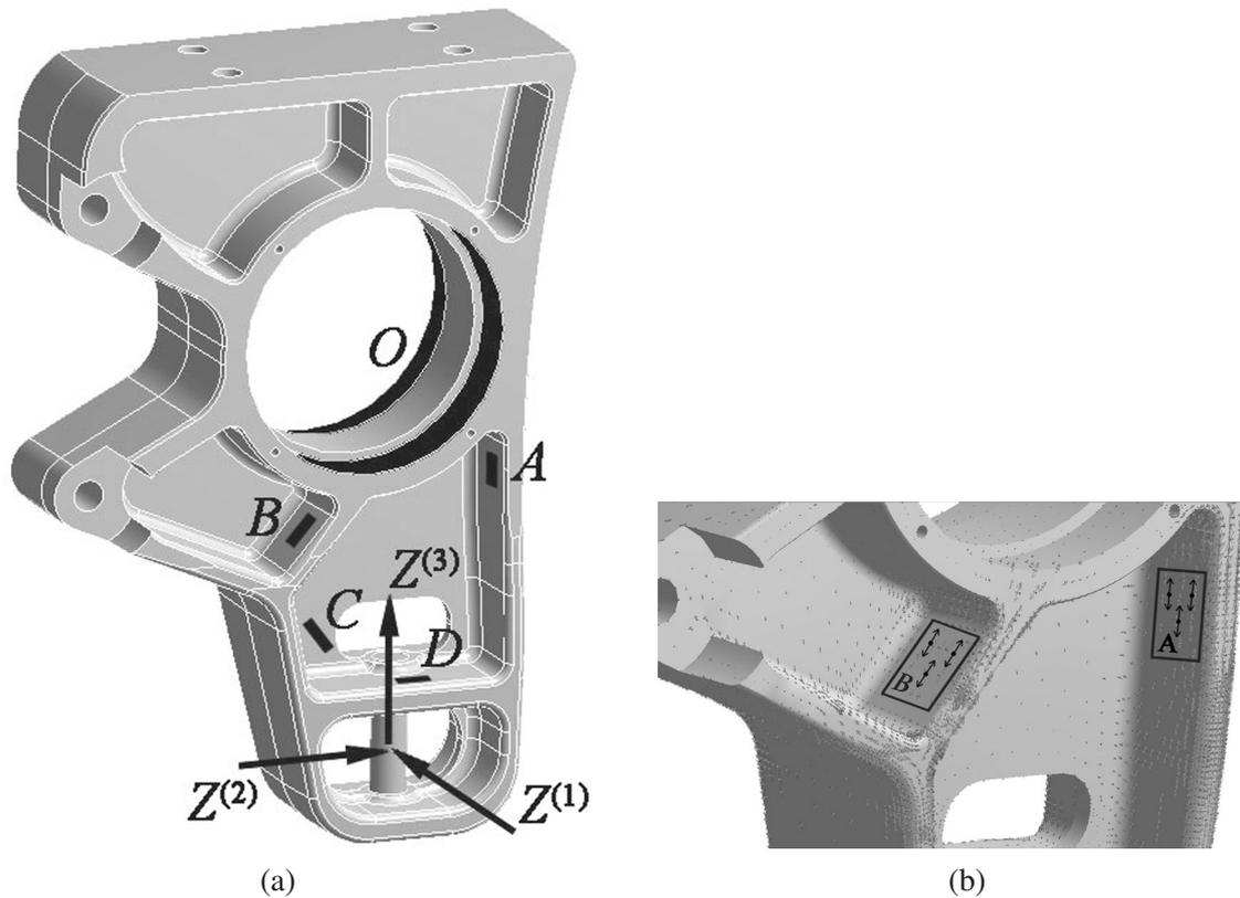
Fig. 5. Structure under investigation: (a) scheme of fastening and loading; (b) choosing the orientation of measurement axes of sensors and locations of measurement points
