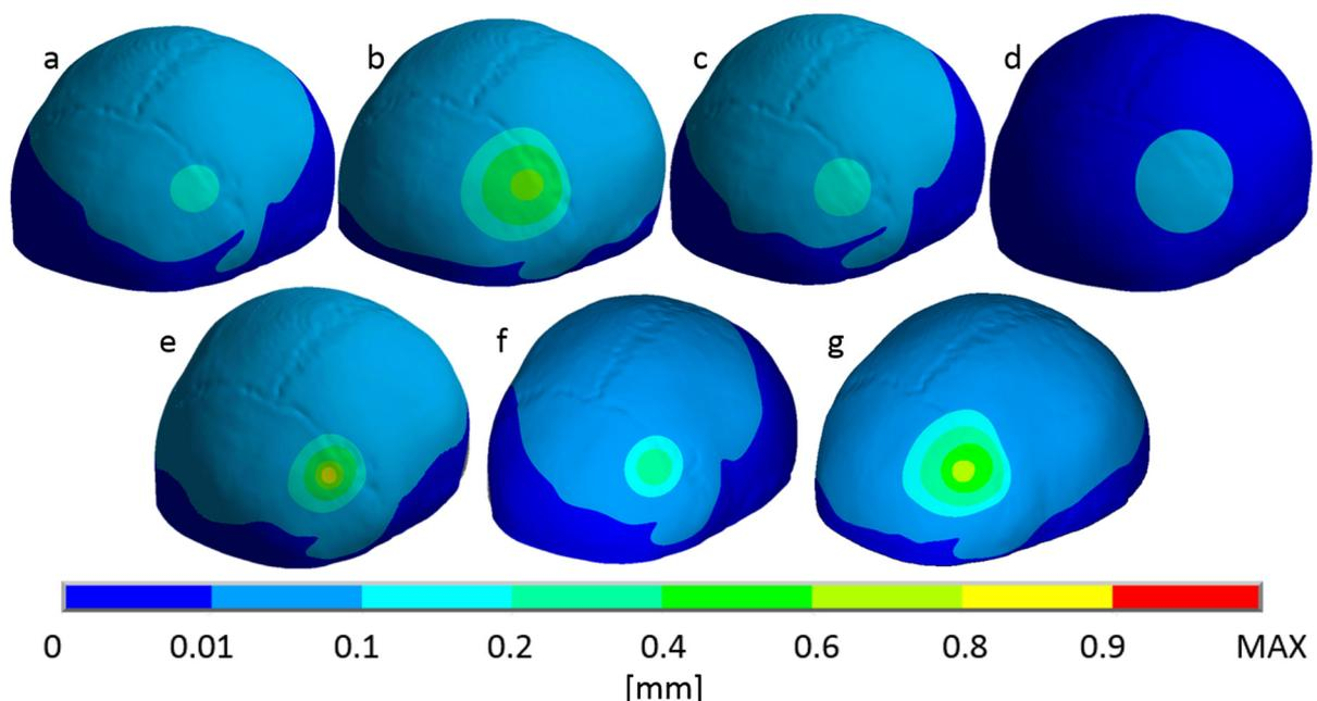
Fig. 5. Distribution of total displacement in all analysed models: a) model **A1**; b) model **A2**; c) model **B**; d) model **C**; e) model **D1**; f) model **D2**; g) model **E**
