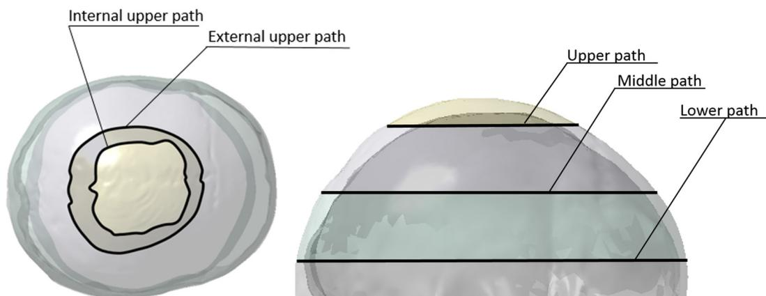
Fig. 7. Paths for evaluation of von Mises strain
