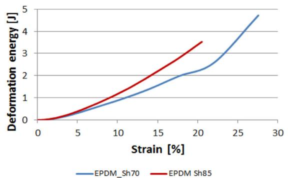
Fig. 6. The deformation energy of the Yeoh models vs. strain for EPDM Sh70 and EPDM Sh85 rubbers – temperature  $-20^{\circ}\text{C}$ , excitation frequency 2 Hz
