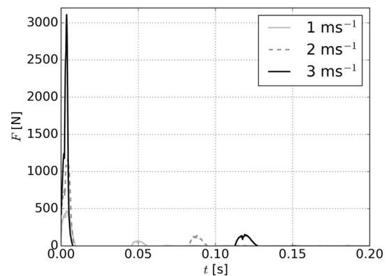
Fig. 4. Force during impact test
