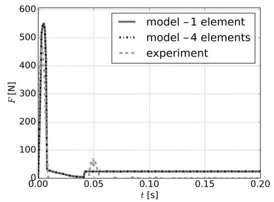
Fig. 10. Comparison of force response of identified model and impact test for  $1 \text{ ms}^{-1}$
