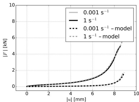
Fig. 15. Comparison of identified model and compression test
