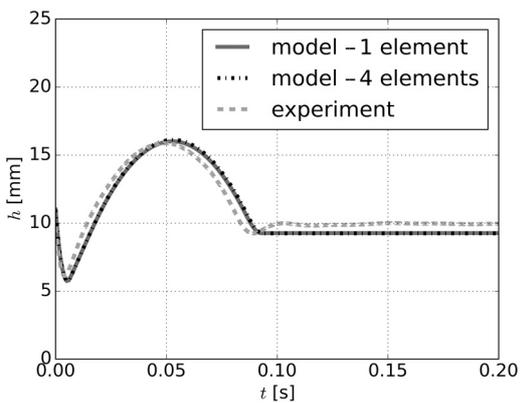
Fig. 11. Comparison of displacement of identified model and impact test for  $2 \text{ ms}^{-1}$
