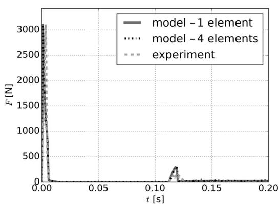
Fig. 14. Comparison of force response of identified model and impact test for  $3 \text{ ms}^{-1}$
