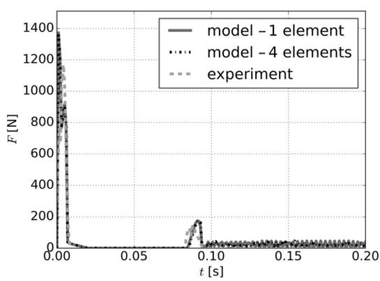
Fig. 12. Comparison of force response of identified model and impact test for  $2 \text{ ms}^{-1}$
