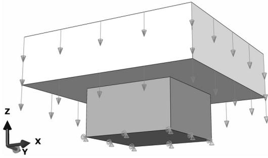
Fig. 5. Model of impact test – 1 element
