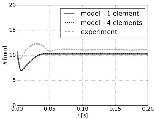
Fig. 9. Comparison of displacement of identified model and impact test for  $1 \text{ ms}^{-1}$
