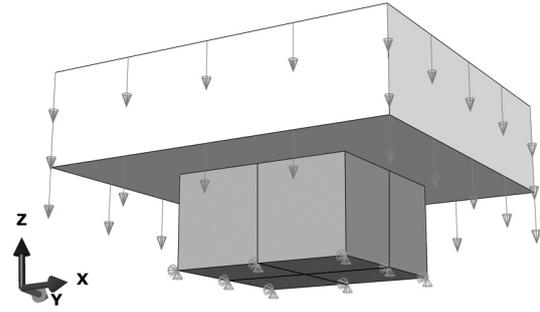
Fig. 6. Model of impact test – 4 elements
