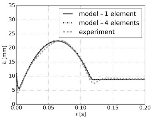
Fig. 13. Comparison of displacement of identified model and impact test for  $3 \text{ ms}^{-1}$
