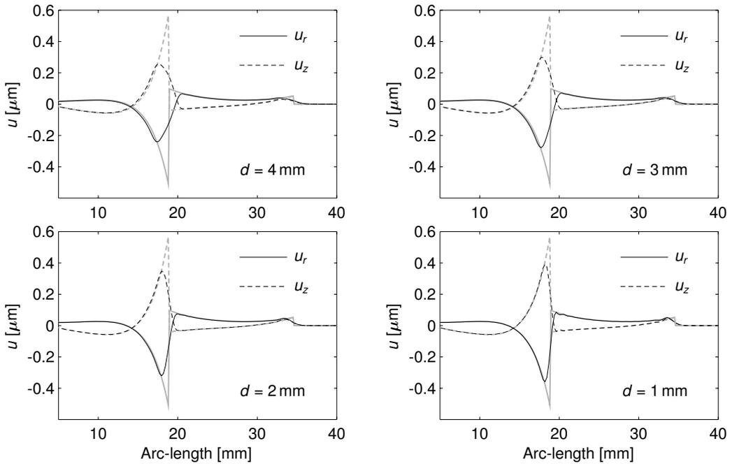
Fig. 11. Comparison of displacements for a FE model to an analytical solution for the cylindrical dipole source with the time function A at time  $6 \mu\text{s}$  over the line  $L$  for particular arm lengths  $d$ . Analytical: gray; FEM: black
