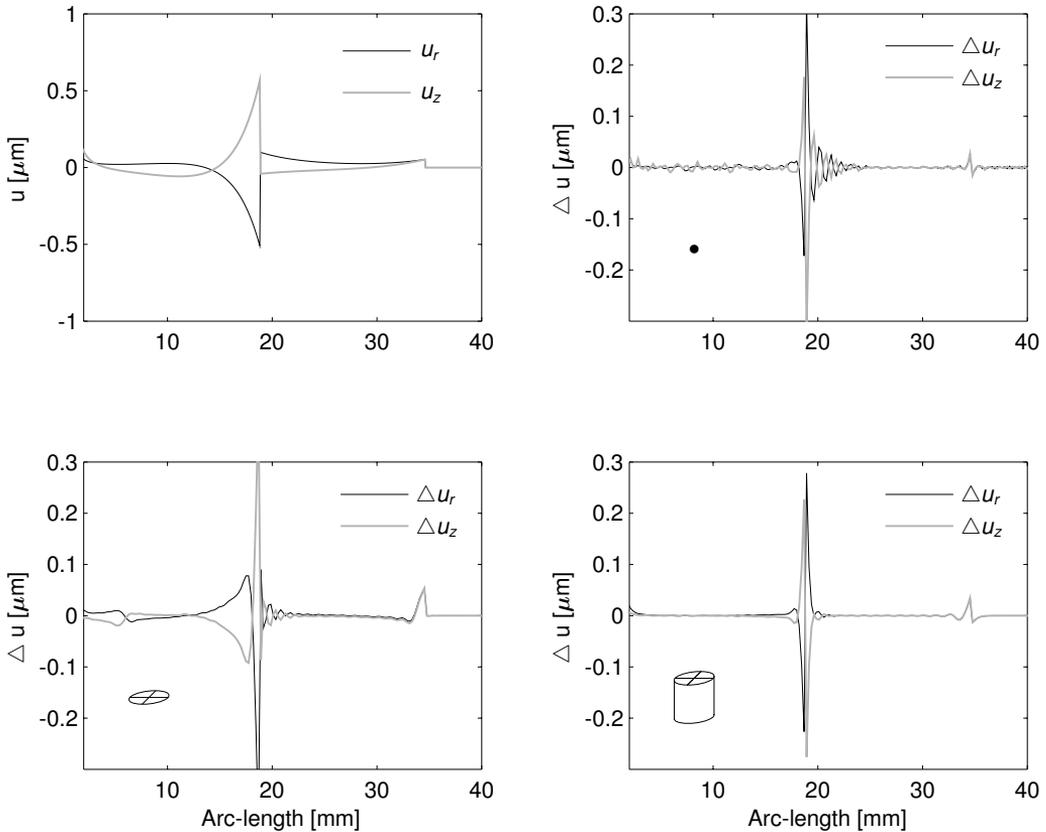
Fig. 10. Comparison of radial ( $u_r$ ) and vertical ( $u_z$ ) displacements for FE-axisymmetric models to an analytical solution for the time function type A at time  $6 \mu\text{s}$  over the line  $L$ . Upper left: analytical solution; the others: absolute errors of FE-solution for particular sources: point, circle area and cylinder
