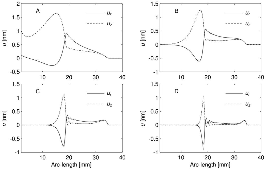
Fig. 7. Comparison of displacements for a FE model to an analytical solution for the circle source with the time function A, B, C, and D at time  $6 \mu\text{s}$  over the line  $L$ . Analytical: gray; FEM: black
