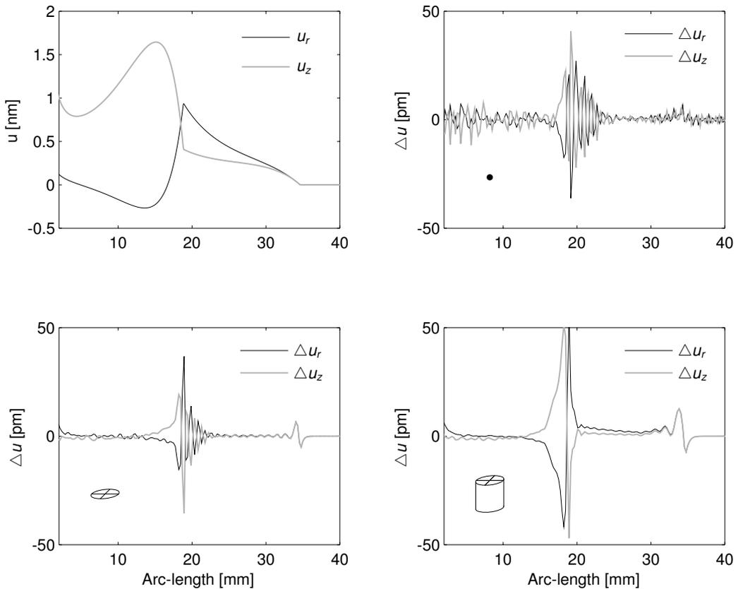
Fig. 6. Comparison of radial ( $u_r$ ) and vertical ( $u_z$ ) displacements for FE-axisymmetric models to an analytical solution for the time function type A at time  $6 \mu s$  over the line  $L$ . Upper left: analytical solution; the others: absolute errors of FE-solution for particular sources: point, circle area and cylinder
