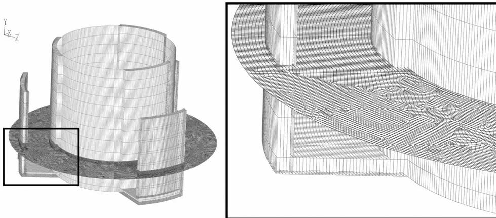
Fig. 5. Detailed view of surface mesh around spacer
