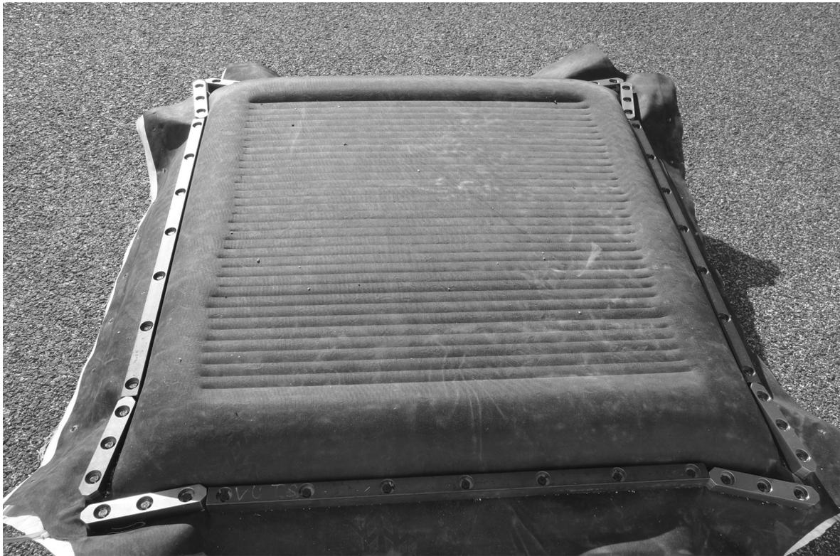
Fig. 4. Panel used in tests in fully inflated condition
