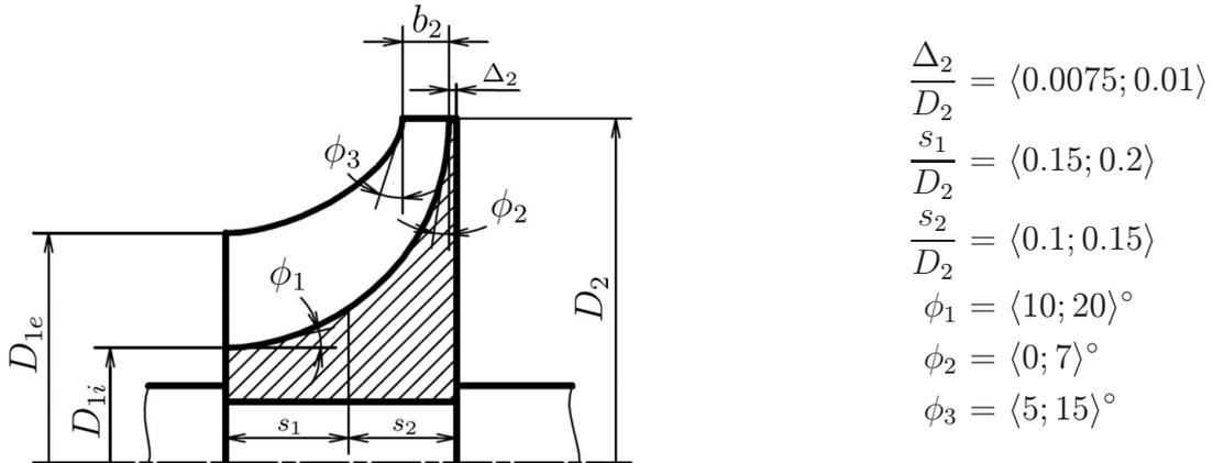
Fig. 2. Impeller geometry, recommended spans are taken from [14]
