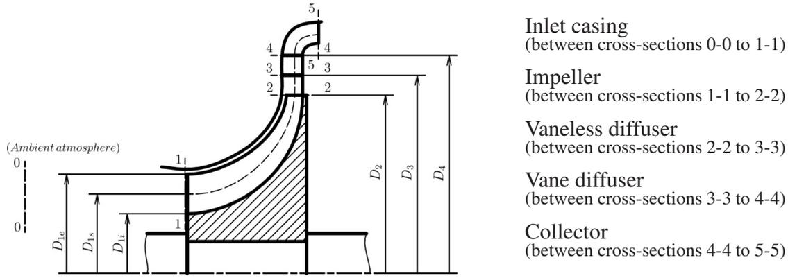
Fig. 1. Radial compressor sketch
