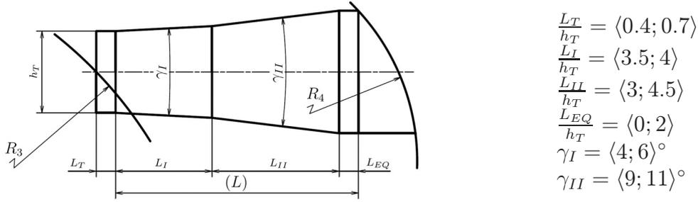
Fig. 3. Diffuser vane geometry, recommended spans are taken from [14]
