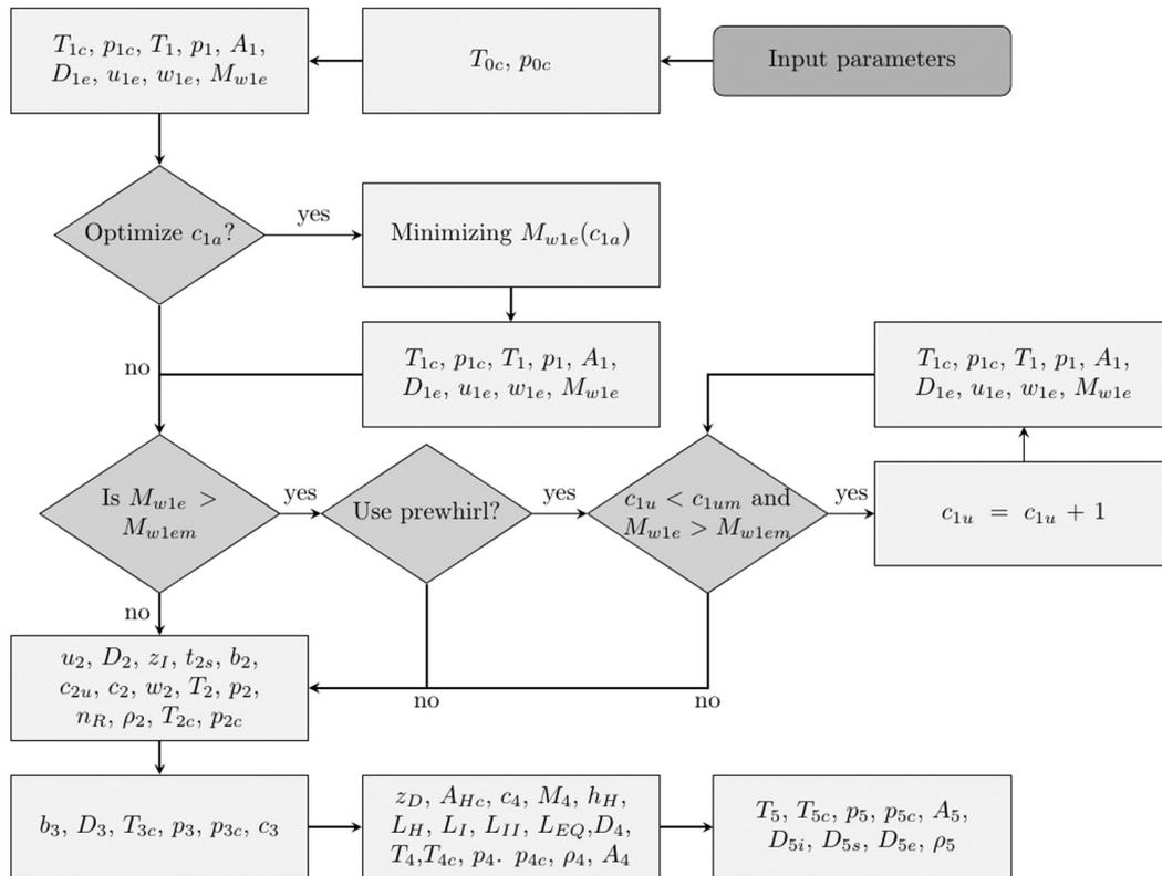
Fig. 4. Flowchart of the design algorithm
