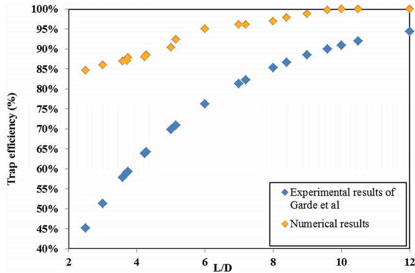
Fig. 11. Comparison of trap efficiencies versus  $L/D$  calculated through experimental data [8] and numerical results
