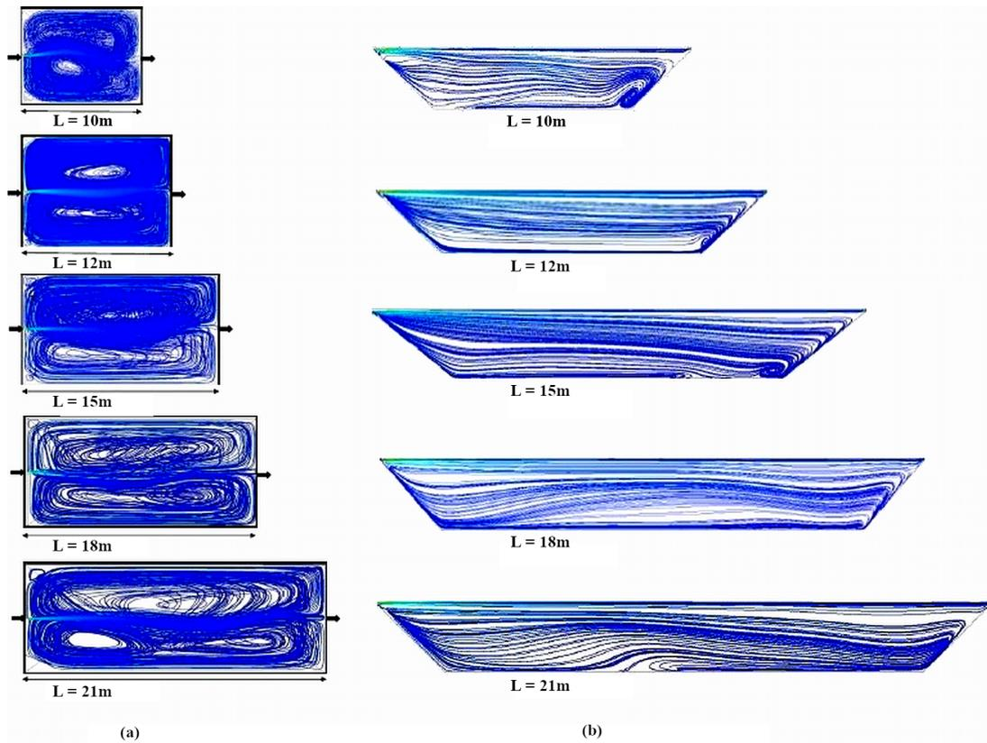
Fig. 4. Streamlines depicted in irrigation basins of different lengths: a) plan view, b) plan of the flow direction
