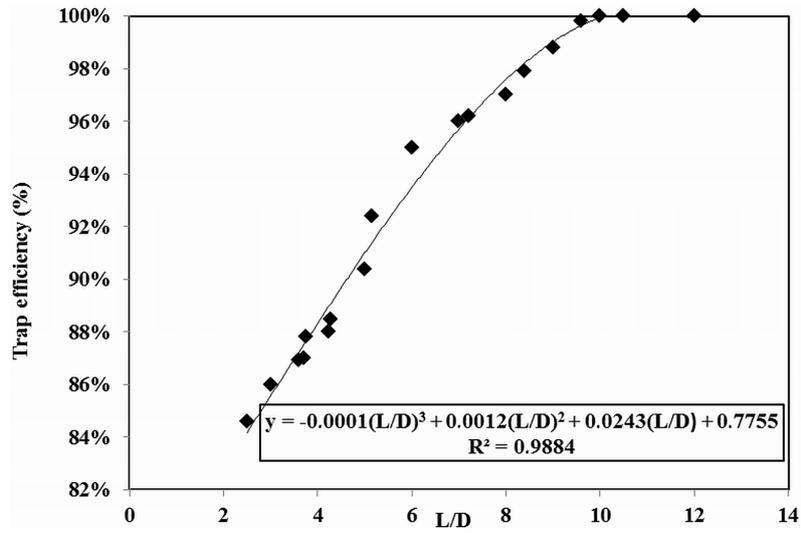
Fig. 12. Trap efficiency versus  $L/D$
