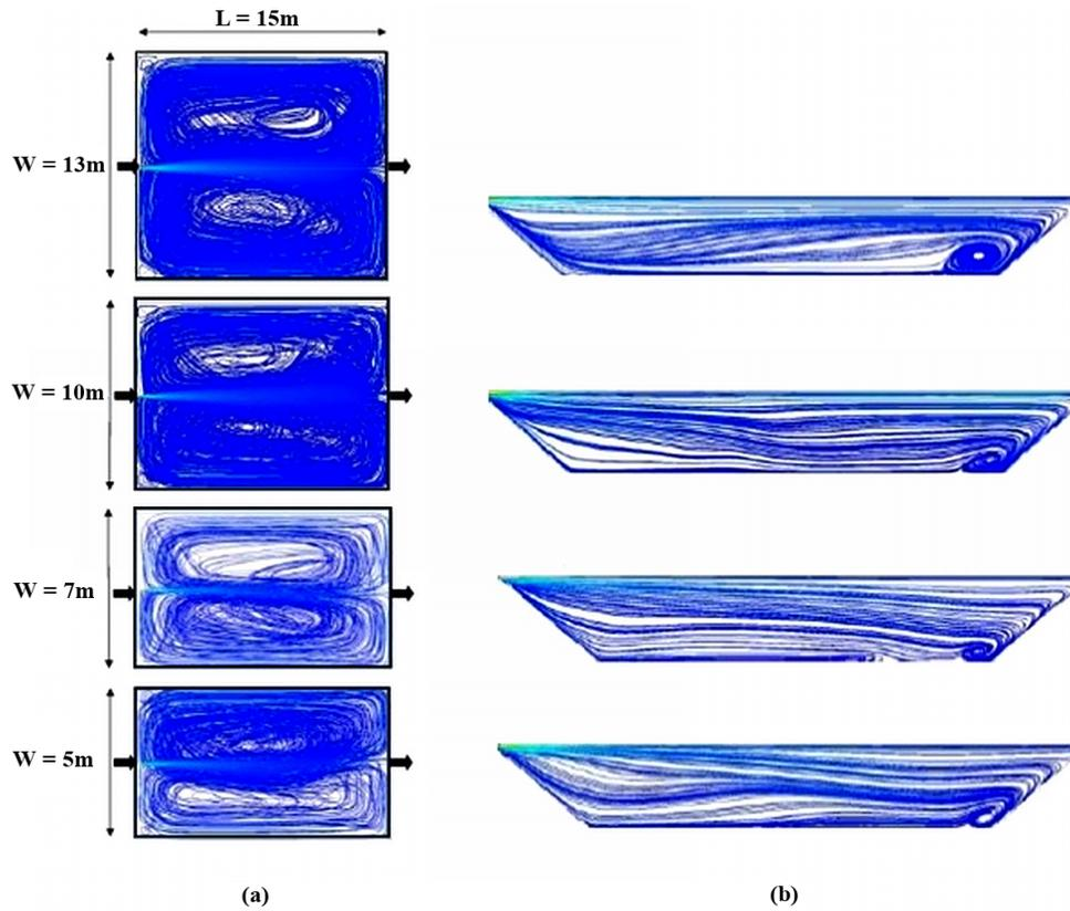
Fig. 6. Streamlines depicted in irrigation basins of different widths: a) plan view, b) plan of the flow direction
