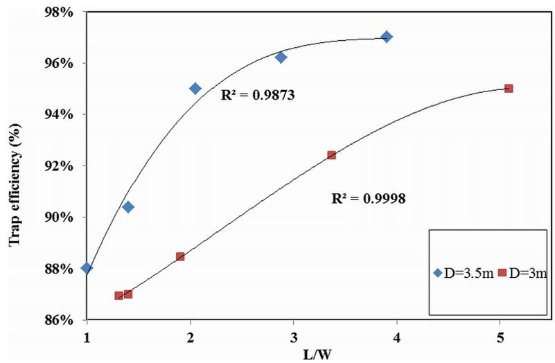
Fig. 14. Trap efficiency versus  $L/W$  for two depth values
