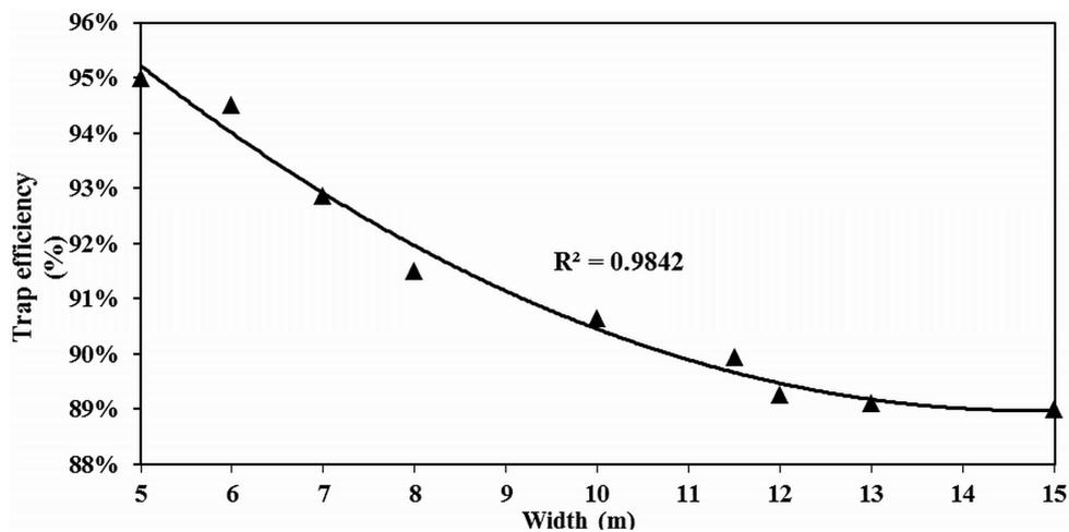
Fig. 7. Trap efficiency versus irrigation basin width
