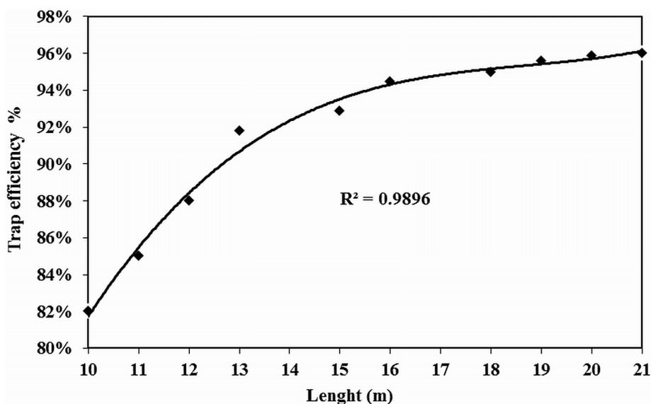
Fig. 5. Trap efficiency versus irrigation basin length
