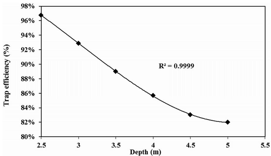
Fig. 10. Trap efficiency versus irrigation storage basin depth
