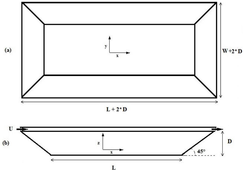
Fig. 1. Specific design of an irrigation storage basin: a) top view, b) side view
