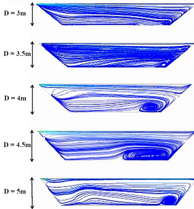
Fig. 9. Streamlines for geometries of different depths depicted in the flow direction
