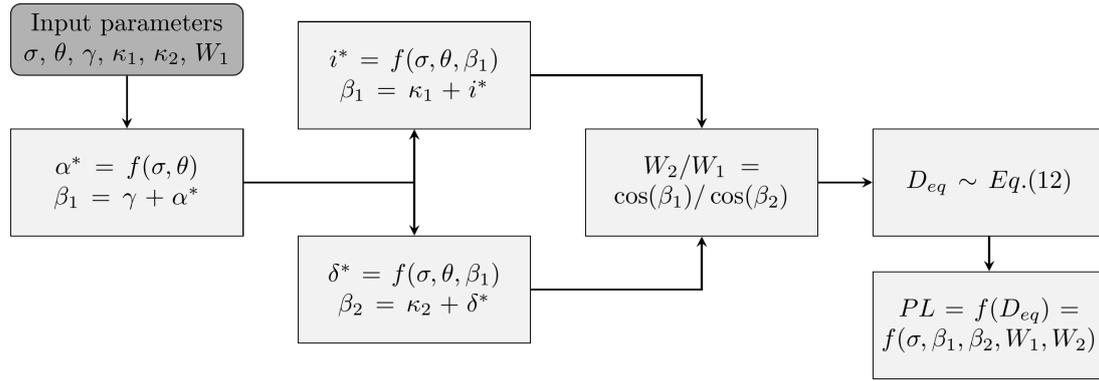
Fig. 4. Workflow for flow parameters prediction
