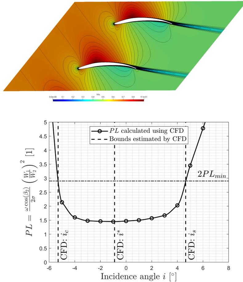
Fig. 2. CFD post processing: (top) flow field example, (bottom) design point finding
