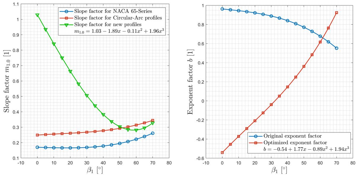
Fig. 5. Optimized functions: (left) slope factor  $m_{1,0}$ , (right) exponent factor  $b$
