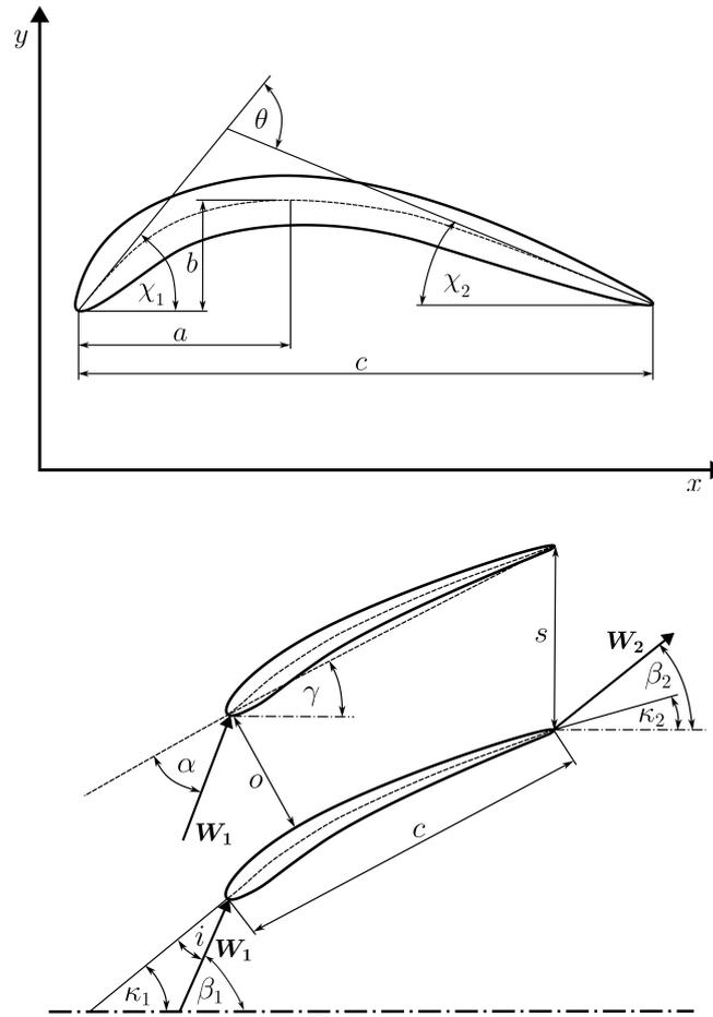
Fig. 1. Cascade nomenclature: (top) profile parameters, (bottom) cascade and flow parameters
