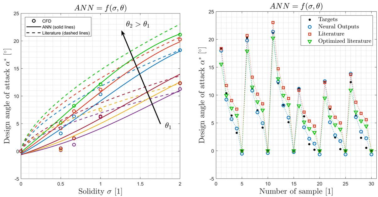
Fig. 7. Results: (left) design angle of attack  $\alpha^*$  correlation comparison in the  $\{\sigma, \theta\}$  space, (right) design angle of attack  $\alpha^*$  correlation comparison against the number of samples
