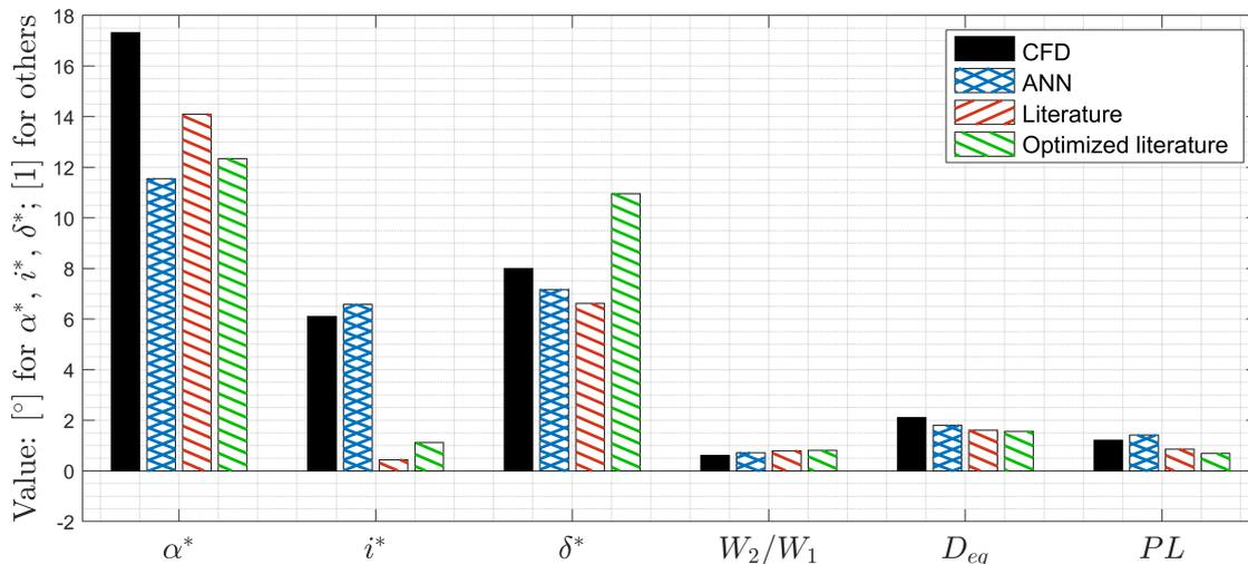
Fig. 9. Comparison of flow field parameters obtained by CFD, ANN and literature correlations performed on the profile excluded from the training data set
