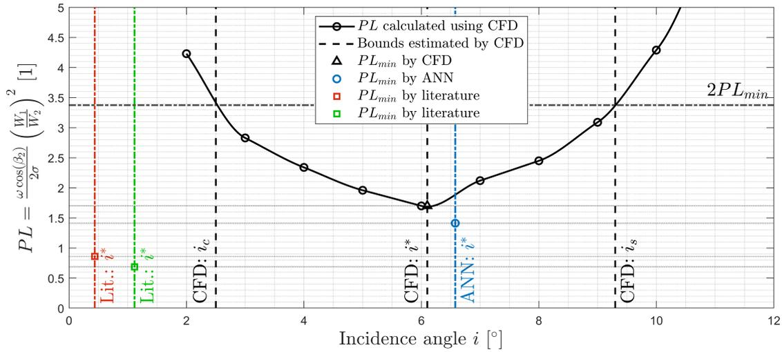
Fig. 10. Design incidence angle  $i^*$  and total pressure loss  $PR$  predictions comparison for the profile excluded from the training data set
