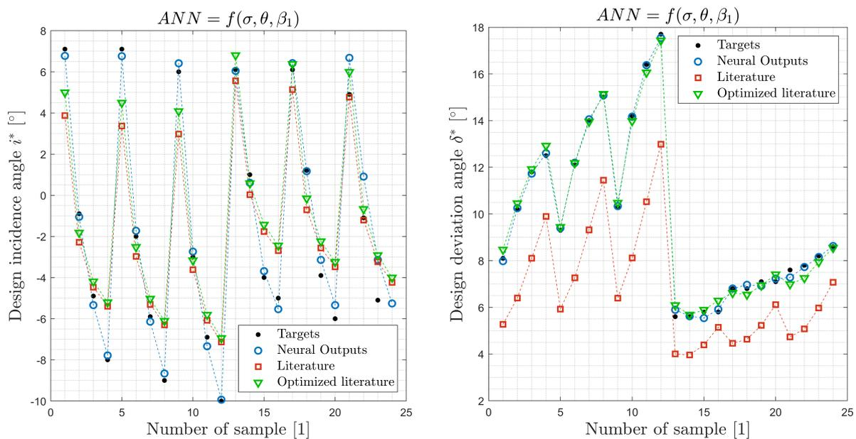
Fig. 8. Results: (left) design incidence angle  $i^*$  correlation comparison, (right) design deviation angle  $\delta^*$  correlation comparison
