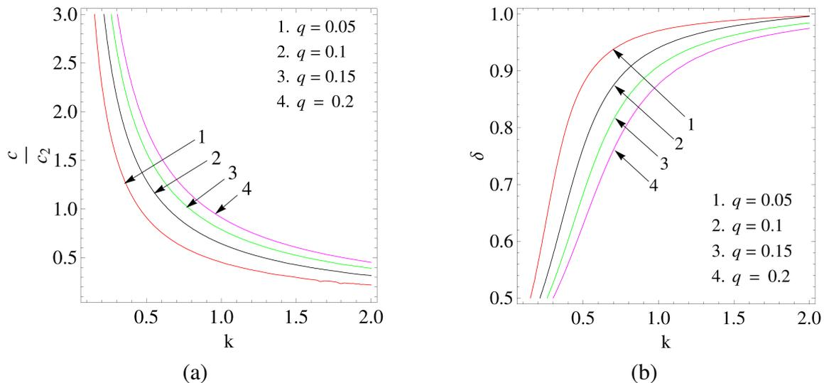
Fig. 6. Variation of (a) phase velocity and (b) attenuation coefficient against the wave number for the thermally conducting parameter  $q$  associated with the homogeneous semi-infinite medium
