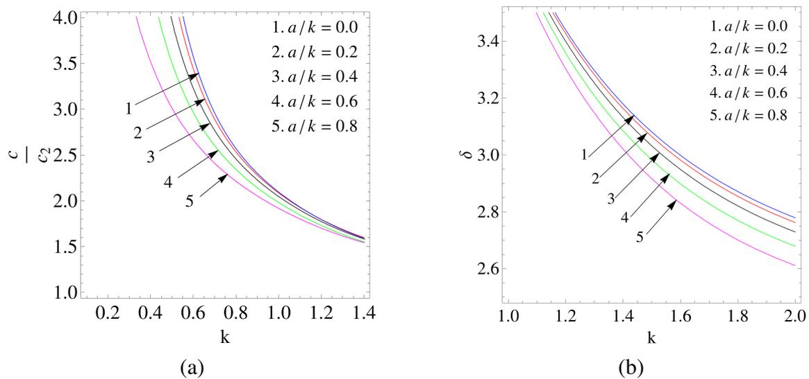
Fig. 2. Variation of (a) phase velocity and (b) attenuation coefficient against the wave number for the gradient parameter  $a/k$  associated with the functionally graded semi-infinite medium
