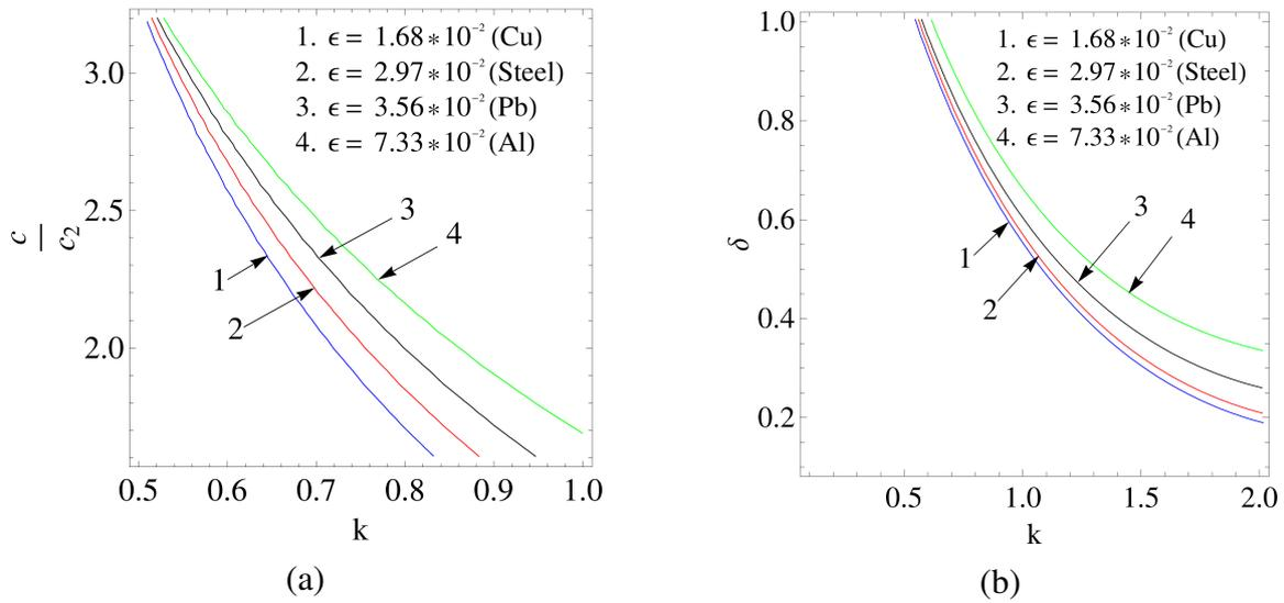
Fig. 3. Variation of (a) phase velocity and (b) attenuation coefficient against the wave number for the coupling coefficient  $\epsilon$  associated with the functionally graded semi-infinite medium
