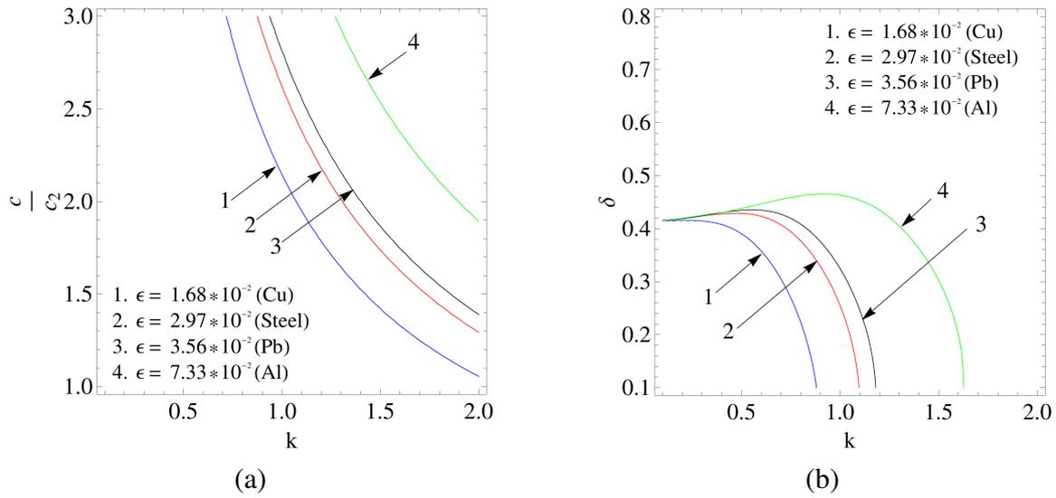
Fig. 5. Variation of (a) phase velocity and (b) attenuation coefficient against the wave number for the coupling coefficient  $\epsilon$  associated with the homogeneous semi-infinite medium
