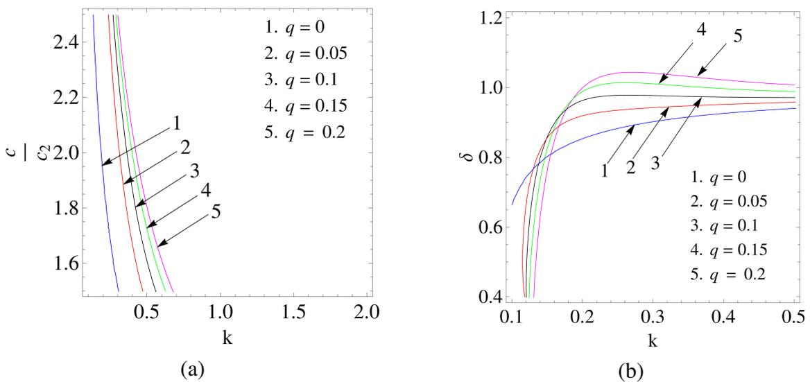
Fig. 4. Variation of (a) phase velocity and (b) attenuation coefficient against the wave number for the thermally conducting parameter  $q$  associated with the functionally graded semi-infinite medium
