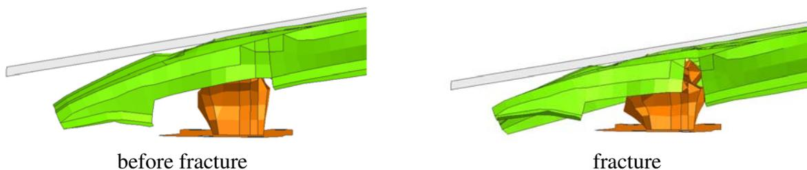
Fig. 15. Fracture on the original steel bumper reinforcement
