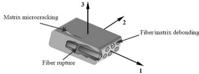
Fig. 3. Composite ply damages
