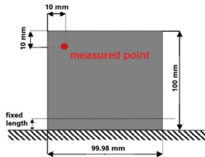
Fig. 5. Basic dimensions of composite plate
