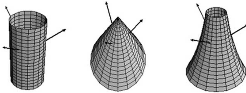
Fig. 10. Comparison of yield surfaces in principal stress coordinates. From left to right: von Mises plasticity, Drucker Prager model, new constitutive model
