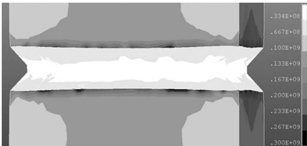
Fig. 5. Plot of the von Mises stress [Pa] at a tensile stress of 100 MPa. Solder gap size: 300\ \mu\text{m}
