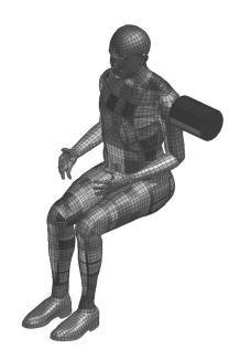
Fig. 5. Shoulder validation setup [1]
