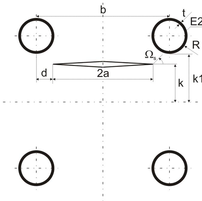
Fig. 1. The geometry of the 2D model used for estimation of micro crack behaviour in the studied particulate composite.
