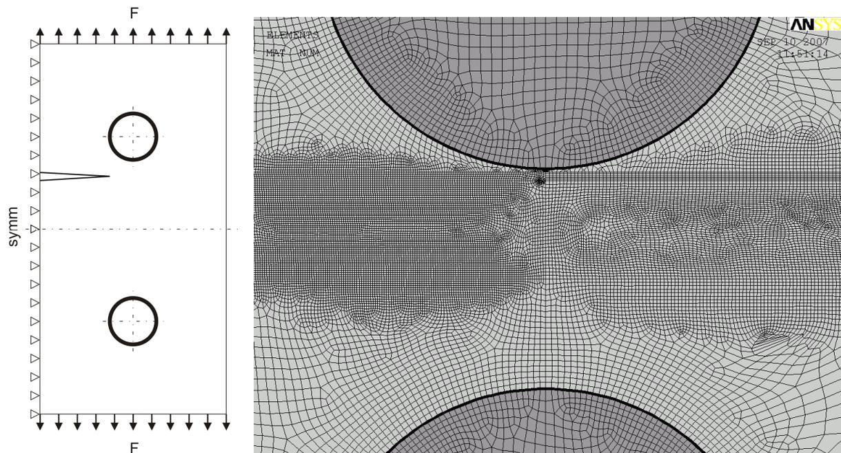
Fig. 2. Schematic representation of FEM model used for calculation of the stress intensity factor.
