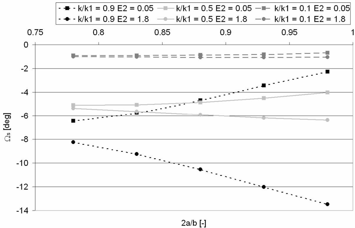
Fig. 4. Dependence of crack propagation direction  $\Omega_s$  on ratio  $2a/b$  for filler volume fraction 35% for variety of ratio  $k/k_1$  and elastic moduli  $E_2$  of interphase.
