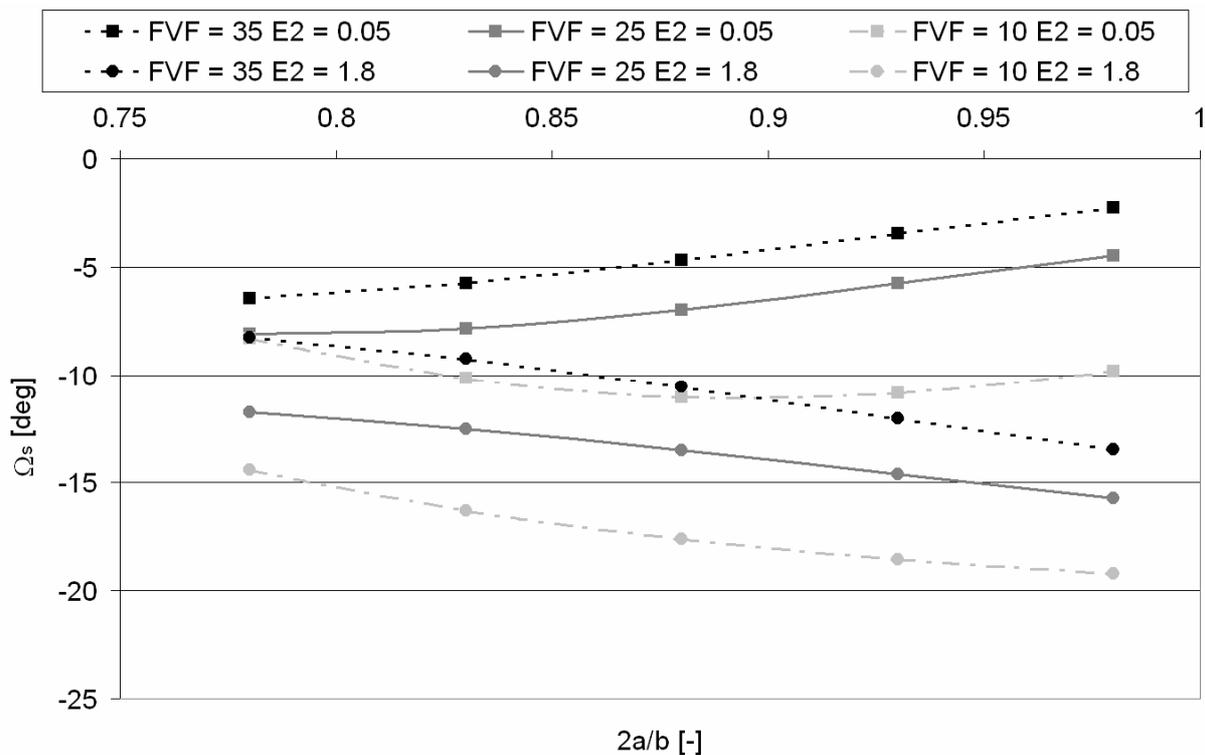
Fig. 3. Dependence of crack propagation direction  $\Omega_s$  on ratio  $2a/b$  for variety of filler volume fraction (FVF) and elastic moduli  $E_2$  of interphase.
